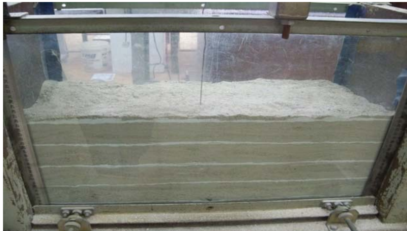
Fig. 11 Initial state of sand before commencement of uplift in loose sand
