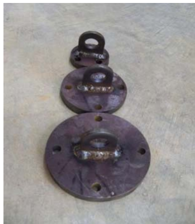
Fig. 4 Symmetrical circular anchor plates at UTM
