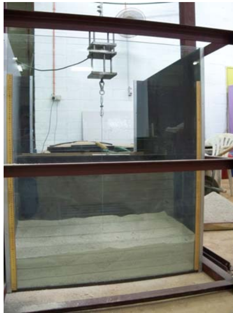
Fig. 5 The setup of uplift test in UTM
