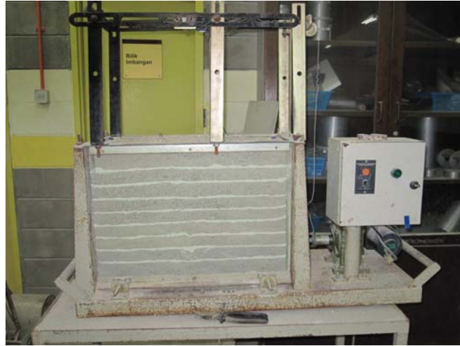
Fig. 6 Set-up of failure mechanism in UTM
