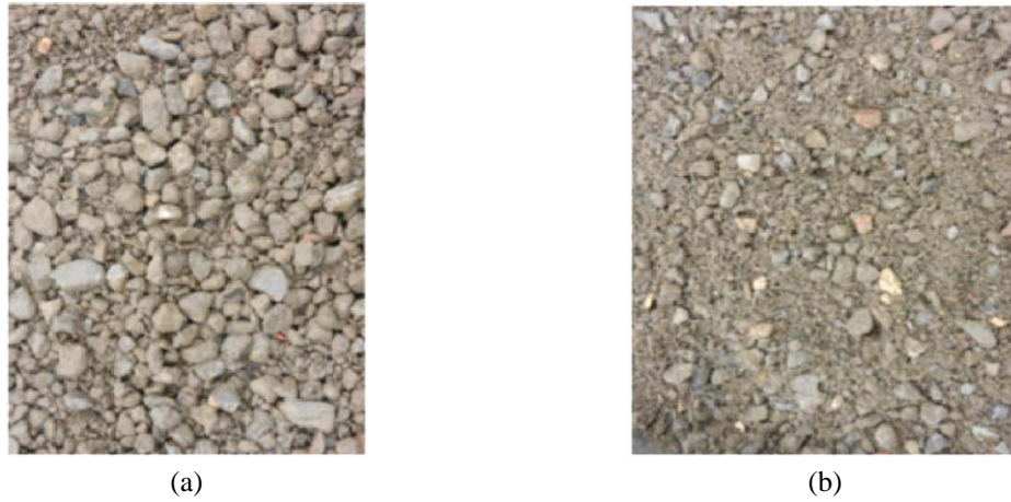
Fig. 1 RCA materials (a) RM001 and (b) RM003
