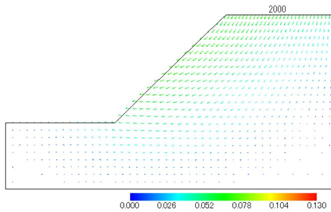
Fig. 14 Displacement vectors of Pubail soil with reinforcement (unit in meter)
