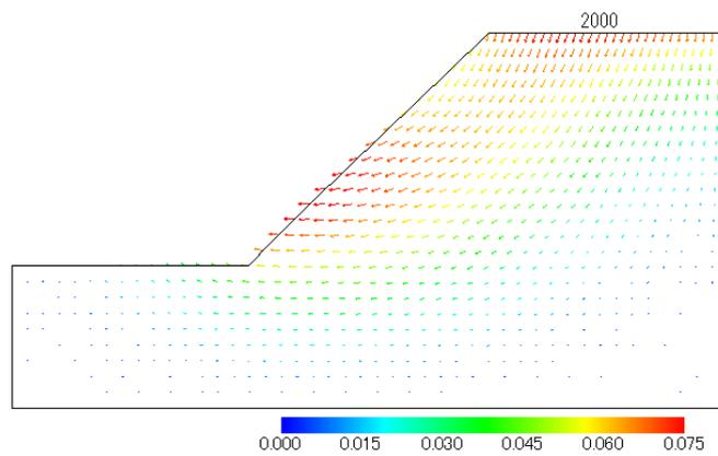
Fig. 15 Displacement vectors of Kuakata soil without reinforcement (unit in meter)
