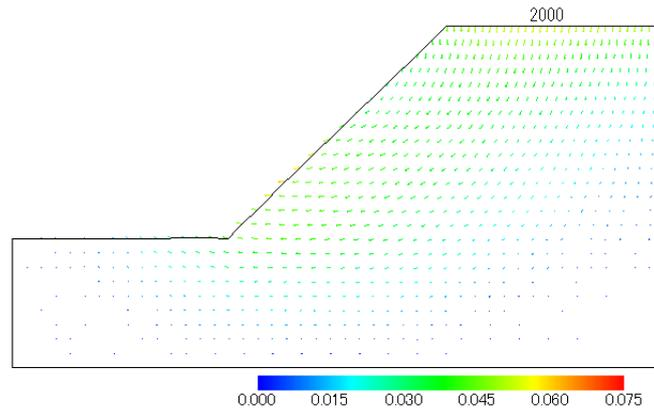
Fig. 16 Displacement vectors of Kuakata soil with vetiver roots (unit in meter)
