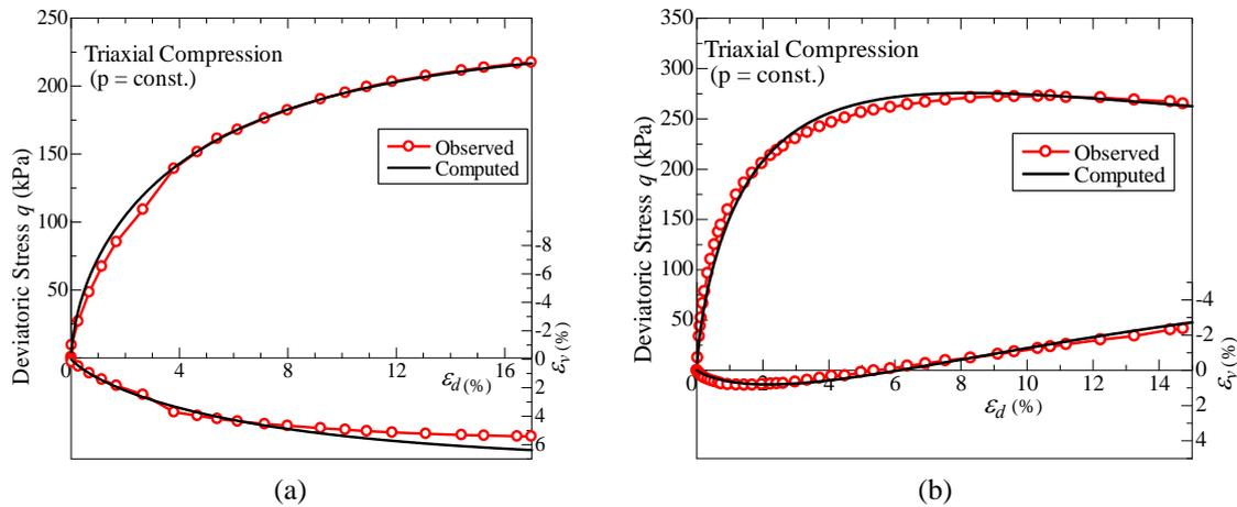
Fig. 3 (a) Observed and computed results of drained triaxial compression tests: (a) Pubail soil; and (b) Kuakata soil
