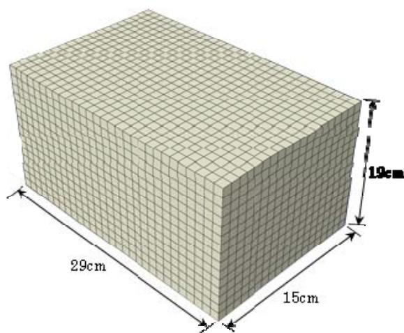
Fig. 6 3D finite element mesh for simulating field shear test
