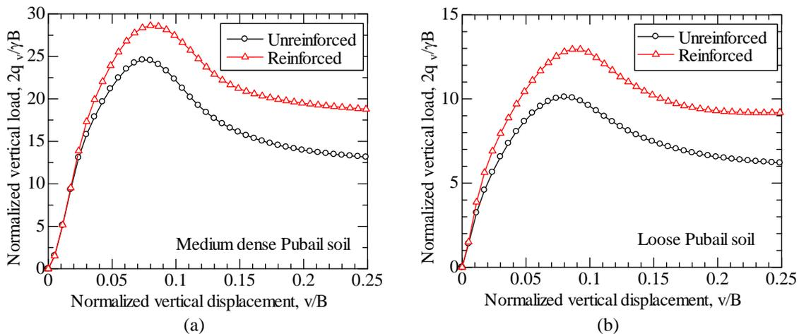
Fig. 9 Normalized vertical load ( $2q_v/\gamma B$ ) vs. normalized vertical displacement ( $v/B$ ) for Pubail grounds: (a) medium dense soils; and (b) loose soils
