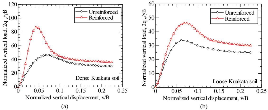
Fig. 10 Normalized vertical load ( $2q_v/\gamma B$ ) vs. normalized vertical displacement ( $v/B$ ) for Kuakata grounds: (a) medium dense soils; and (b) loose soils
