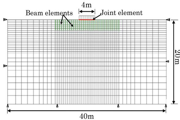
Fig. 8 Finite element mesh for bearing capacity analyses
