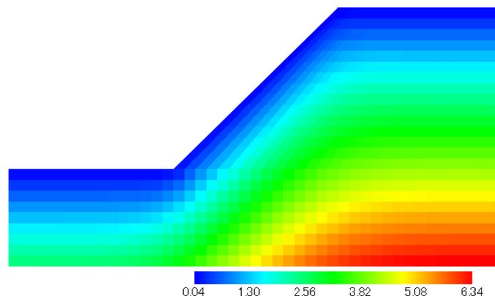
Fig. 12 Effective vertical stress of initial ground: Pubail Soil - unit in ( $\times 9.8 \text{ kPa}$ )
