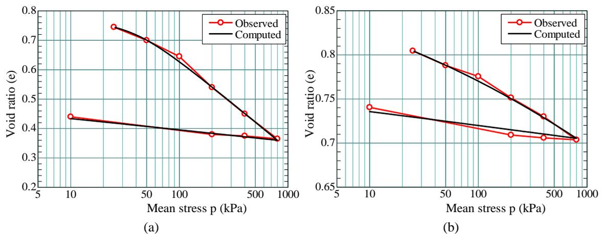
Fig. 2 e-lnp curve obtained from 1-D consolidation tests: (a) Pubail soil and (b) Kuakata soil
