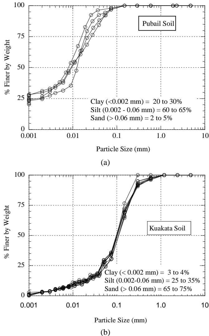
Fig. 1 Particle size distribution: (a) Pubail soil; and (b) Kuakata soil
