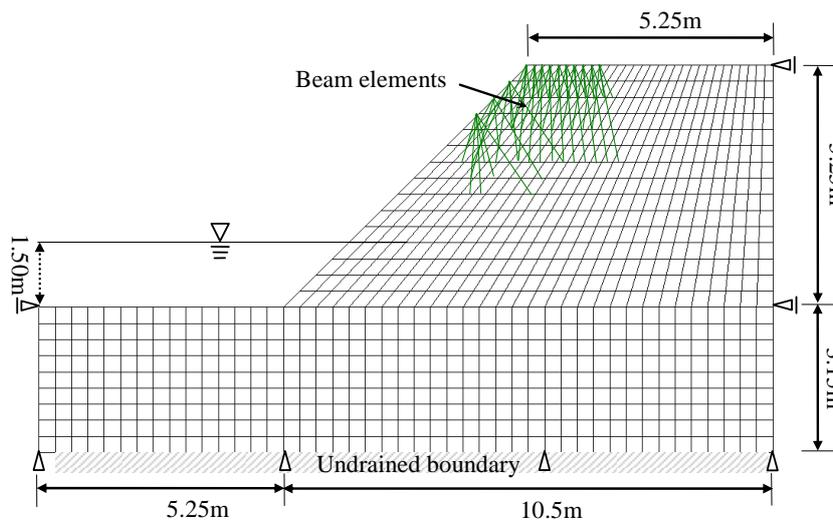
Fig. 11 Finite element mesh for slope stability analyses
