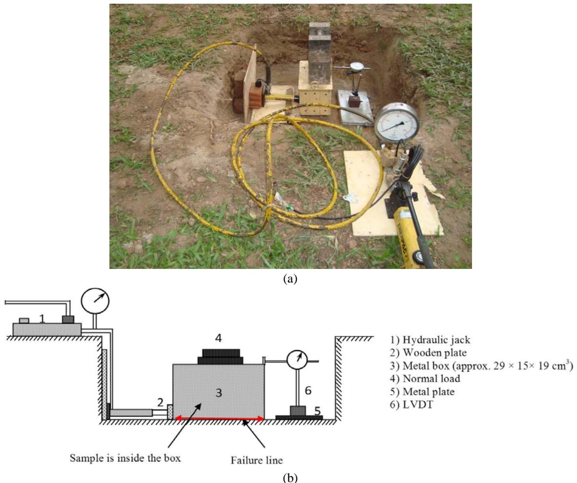
Fig. 4 Experimental set-up for field test: (a) photograph showing the experimental set-up; and (b) schematic diagram showing the experimental set-up
