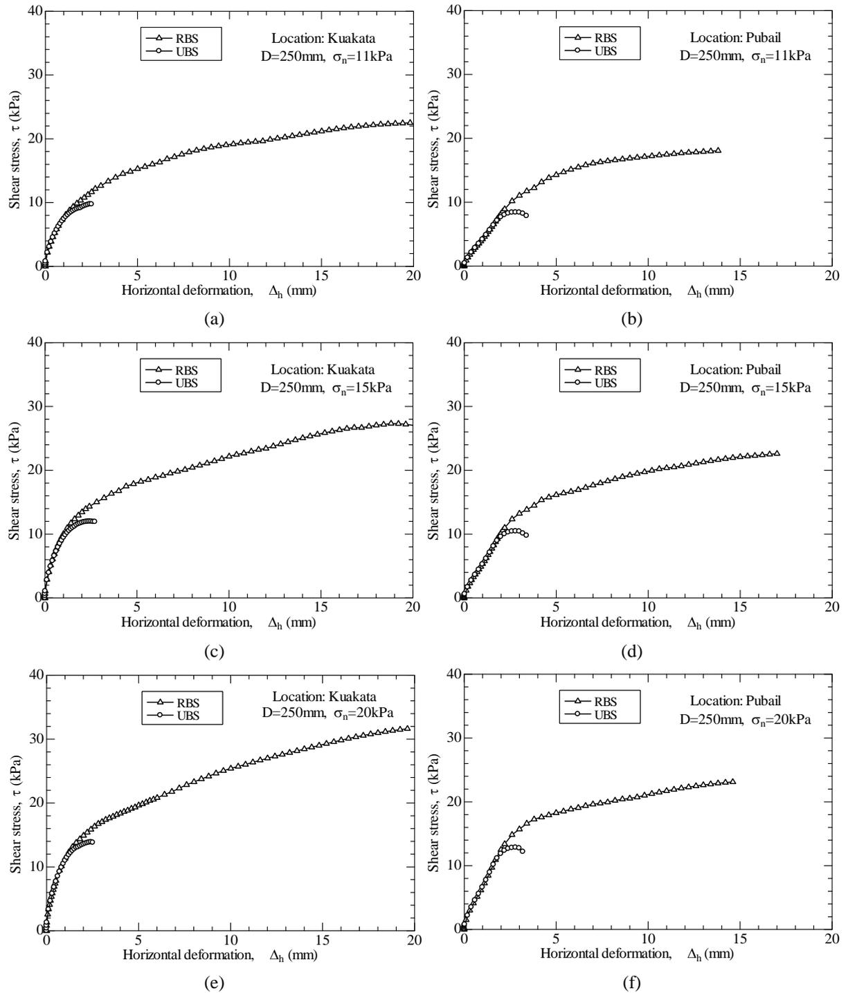
Fig. 7 Simulation of field shear stress vs. horizontal deformation results: (a) Kuakata soil ( $\sigma_n = 11$  kPa); (b) Kuakata soil ( $\sigma_n = 15$  kPa); (c) Kuakata soil ( $\sigma_n = 20$  kPa); (d) Pubail soil ( $\sigma_n = 11$  kPa); (e) Pubail soil ( $\sigma_n = 15$  kPa); (f) Pubail soil ( $\sigma_n = 20$  kPa)
