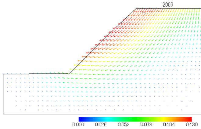
Fig. 13 Displacement vectors of Pubail soil without reinforcement (unit in meter)
