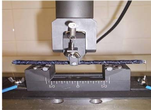
Fig. 5 Setup for characterizing piezoresistive behavior of BCR
