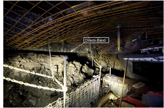
Fig. 8 A coal burst event at Auster Mine, Australia. The coal rib burst out during roadway development. The overburden depth was 550 m (NSW Mine Safety Investigation Unit, 2015).
