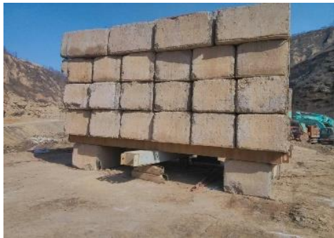
(b) Load test
