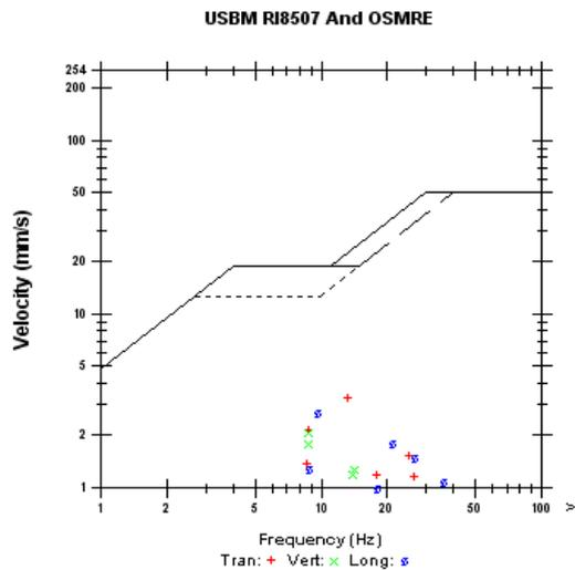
Fig. 1 USBM RI 8507 and OSMRE vibration Standard (Siskind *et al.* 1980). Dashed line illustrates the damage limit level for older homes, plaster on wood lath construction for interior walls. Solid line illustrates the damage limit level for modern homes, drywall interior. Tran (+), Ver (x), Lon (\$) symbol indicate transversal, vertical and longitudinal components of vibration wave, respectively
