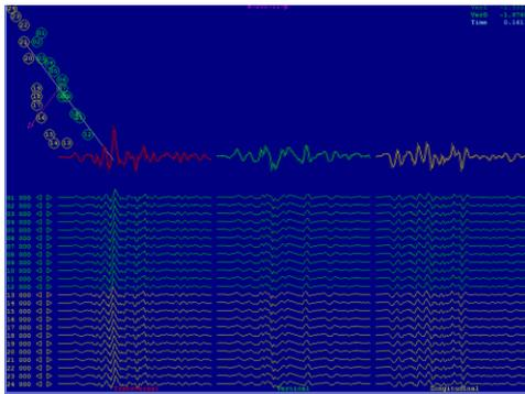
Fig. 15 Blast vibration analysis screen. There are two groups (green and yellow). At this stage no delay applied to the blast holes
