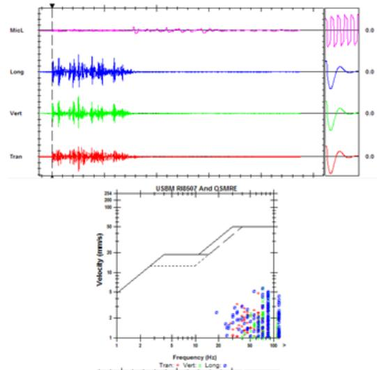
Fig. 8 Event report of blast vibration (20.07.2011) belongs to seismograph:14465
