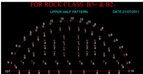
Fig. 11 Blast pattern of the blast at tunnel inlet portal (left tube) (21.07.2011). 1 (5) means: cap no:1 having 5 cartridges: 0.545 kgx4=2.5 kg/ hole. Some holes contain 7 cartridges, 0.545 kgx7=3.5 kg/hole.
