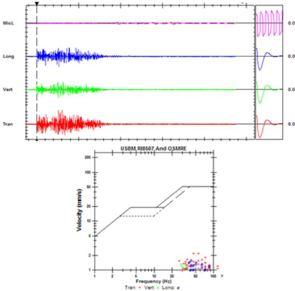
Fig. 10 Event report of blast vibration (20.07.2011) belongs to seismograph:12269
