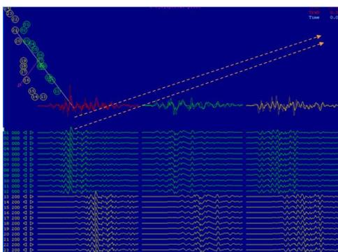
Fig. 16 Blast vibration analysis screen. There are two groups (green and yellow). At this stage 200 ms delay applied to the second group blast holes. Notice the vibration reduction especially at the transversal component (In case of Tran (z): zero delay: vibration is 10.41 unit, in case of Tran (D): 200 ms delay, vibration is 0.32 unit)
