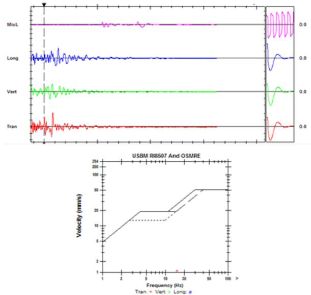
Fig. 6 Serial no: 14465. Event report of the blast at tunnel outlet portal (21.07.2011)
