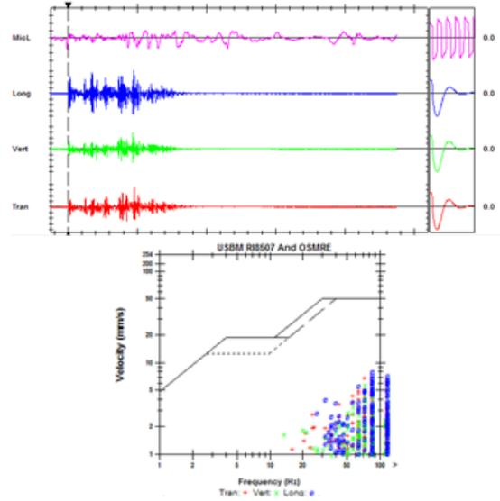
Fig. 12 Event report of blast vibration measured by seismograph 14465
