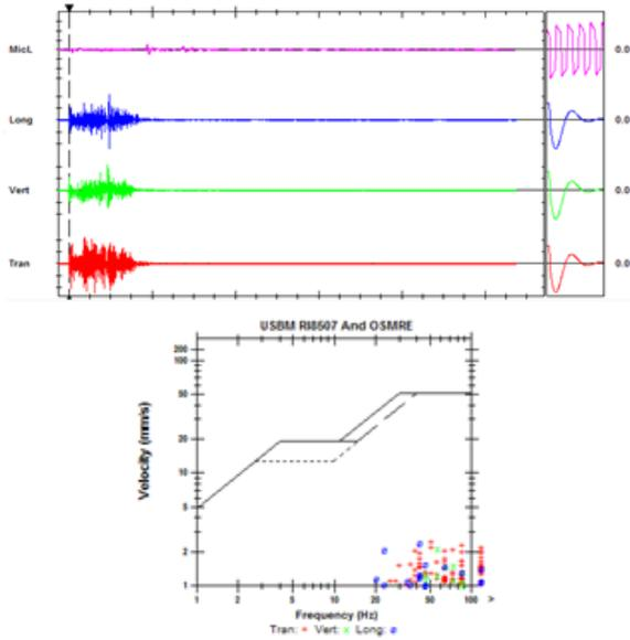
Fig. 14 Event report of blast vibration measured by seismograph 12270
