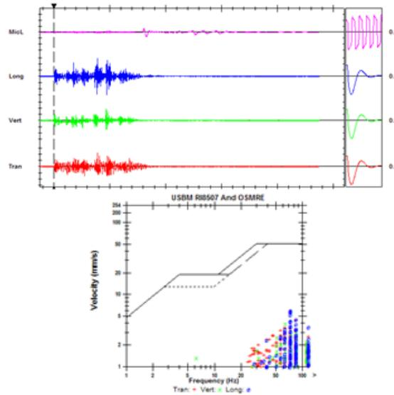
Fig. 13 Event report of blast vibration measured by seismograph 12269
