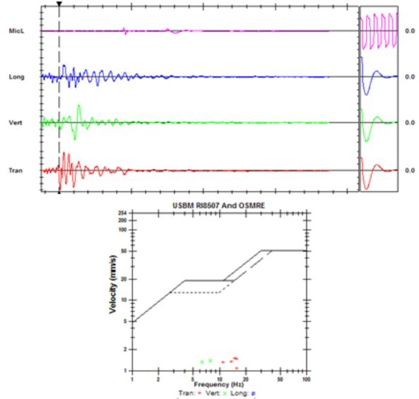
Fig. 4 Event report of the blast at tunnel outlet portal (20.07.2011)
