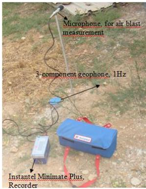
Fig. 2 Instantel Minimate Plus Seismograph with 3-component geophone and microphone
