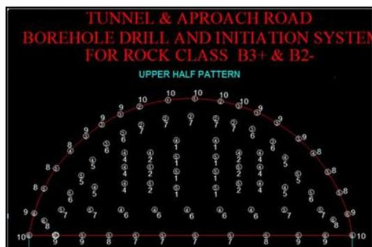
Fig. 7 Blast pattern of the blast at tunnel inlet portal (left tube) (20.07.2011). 1 (4) means: cap no:1 having 4 cartridges: 0.5 kgx4=2 kg/ hole. Some holes contain 5 cartridges, 0.5 kgx5=2.5 kg/hole
