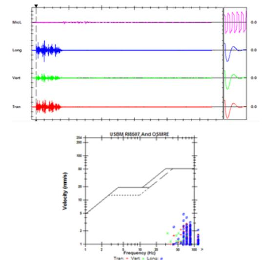
Fig. 9 Event report of blast vibration (20.07.2011) belongs to seismograph:12270
