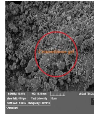
(c) Stabilized marine sand with 20% partial replacement of cement and 5% bentonite
