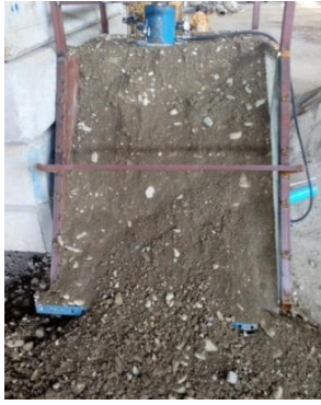
Fig. 7 The unreinforced slope failure
