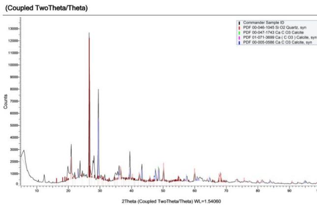
Fig. 2 X-ray diffraction of expansive soil
