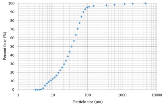
Fig. 1 Grain size distribution curve of clay soil
