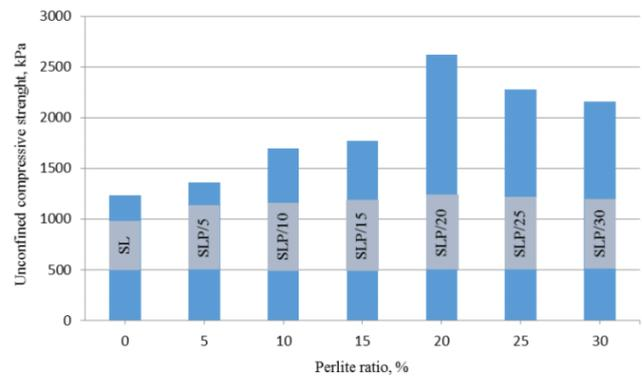
Fig. 11 Unconfined compressive strength after freeze-thaw cycles
