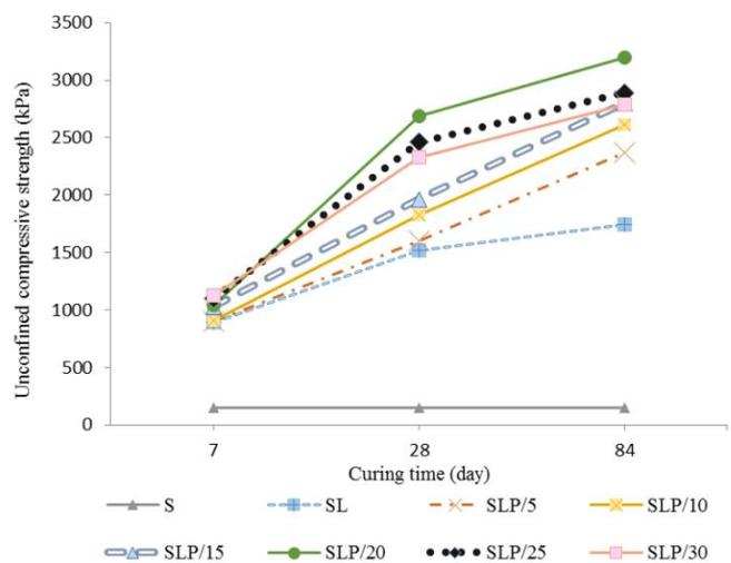
Fig. 9 Unconfined compressive strength of specimens
