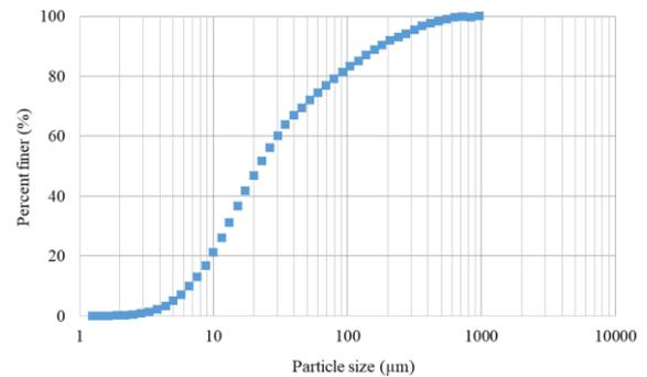
Fig. 3 Grain size distribution curve of hydrated lime
