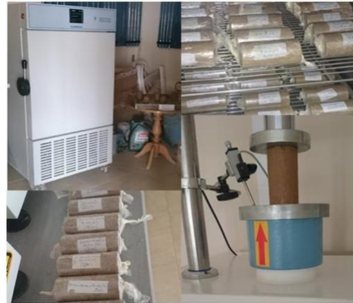
Fig. 10 Close system freezing-thawing cabin and test specimens
