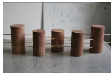
Fig. 2 Bolted red sandstone specimens
