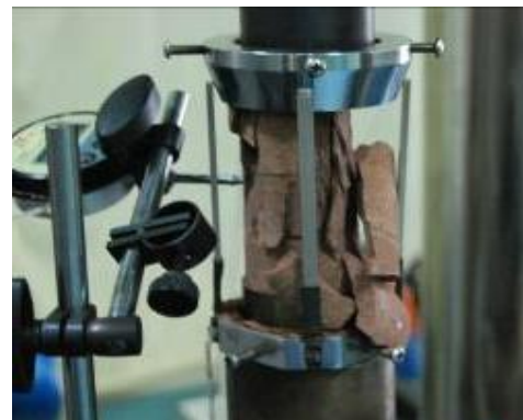
(a) Non-bolted specimen
