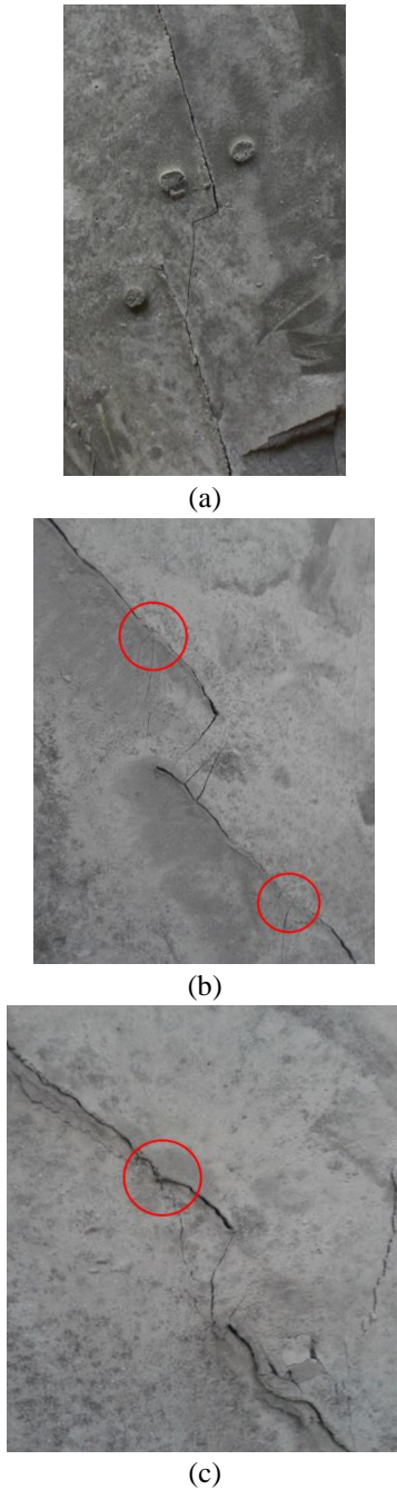
Fig. 20 Asperity “interlocking crack” concept (a) U23 (JRC 4-6, no interlocking crack), (b) U20 (JRC 10-12, shear-tensile interlocking crack) and (c) U5 (JRC 18-20, shear-tensile interlocking crack)
