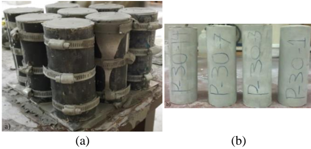
Fig. 2 The preparation of samples using the mold, (a) The mold of sample preparation and (b) The prepared samples
