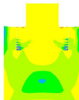
Fig. 9 Static plastic strain of the second method ( $\eta=2.410$ )
