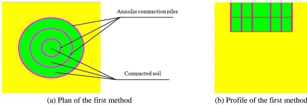
Fig. 2 Simplification of composite foundation by the first simplified method
