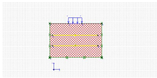
Fig. 5(b) Model for double layers of geocell
