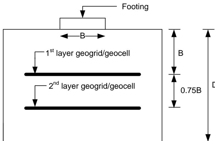
Fig. 3 Typical placement of reinforcement
