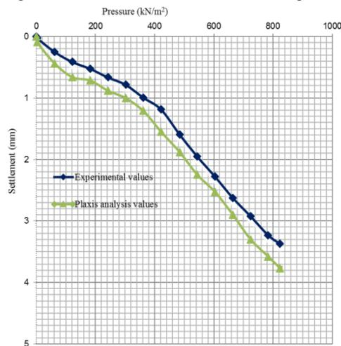
Fig. 7(b) Pressure v/s settlement for double layers of geocell
