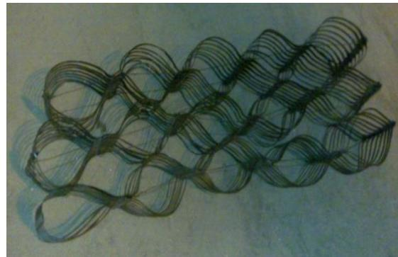
Fig. 1(b) Geocell used in the study
