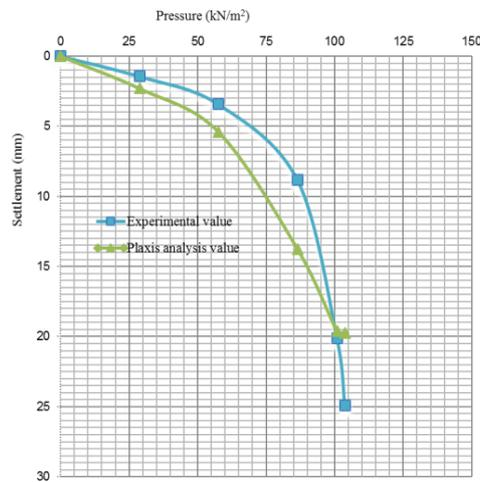
Fig. 7(a) Pressure v/s settlement for virgin soil
