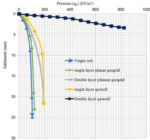
Fig. 4 Pressure v/s settlement curves for unreinforced soil and reinforced soil
