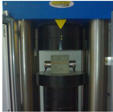
Fig. 4 Uni-axial compression apparatus
