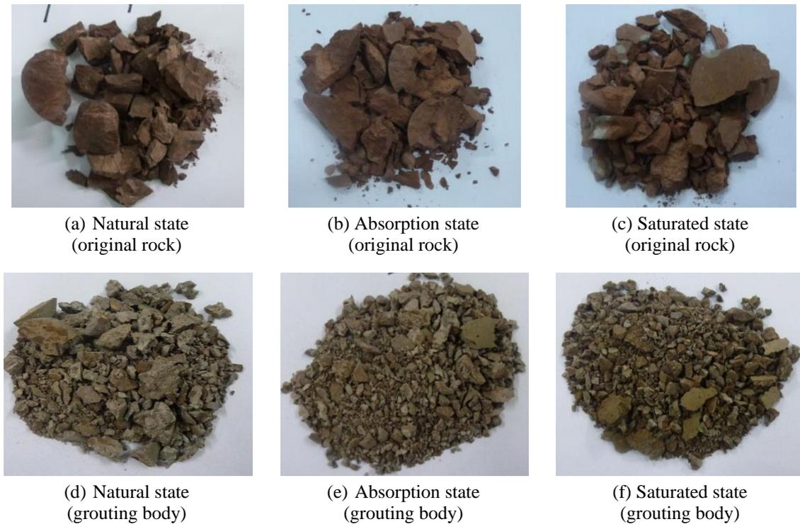
Fig. 4 Failure characters of specimens under different water-bearing states at the same impact velocity
