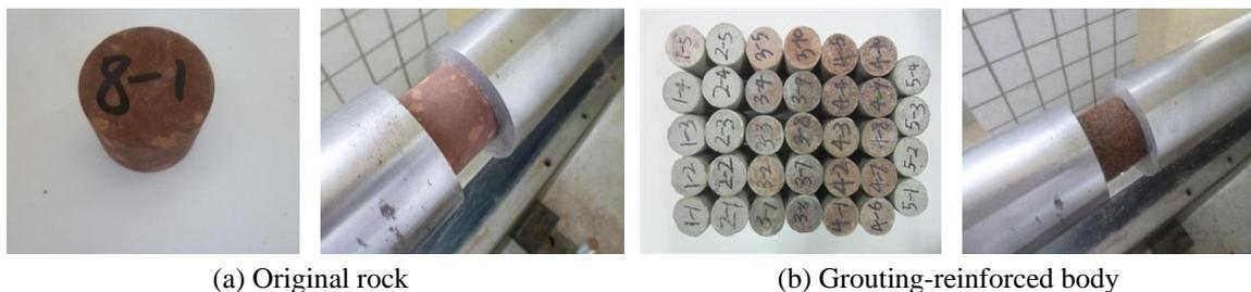
Fig. 1 Specimen preparation
