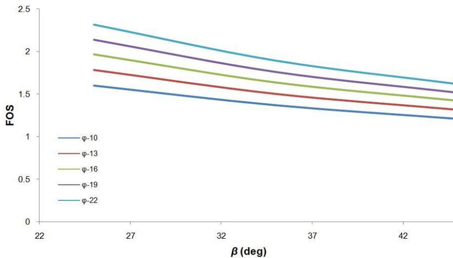
Fig. 5 Relation between stability of slopes and slope angles
