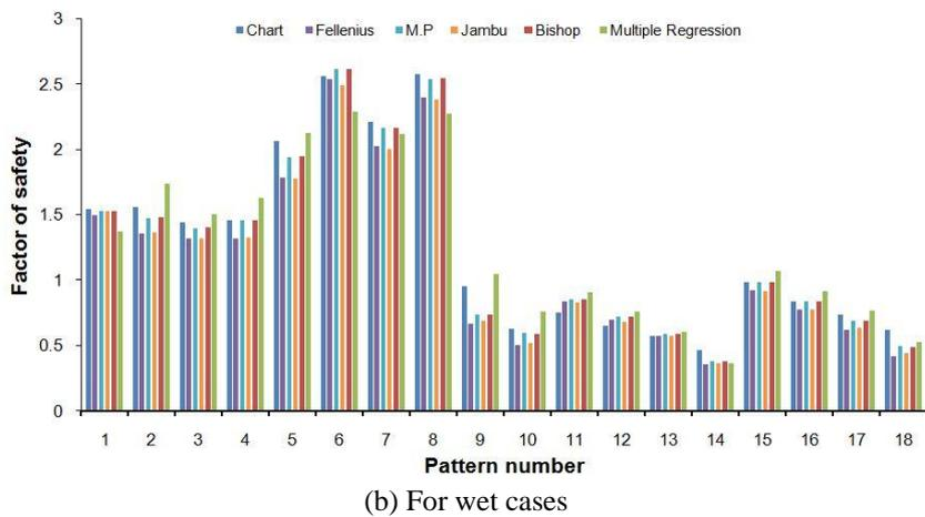
Fig. 15 Variation of the determined factor of safety using different various methods
