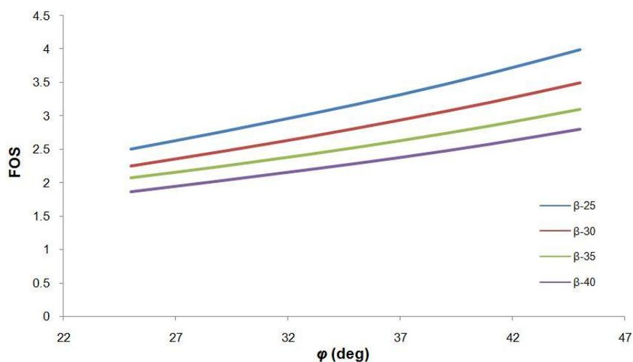
Fig. 2 Relation between stability of slopes and angle of internal friction of soils  $\phi$
