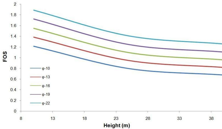
Fig. 4 Relation between stability of slopes and height of the soils
