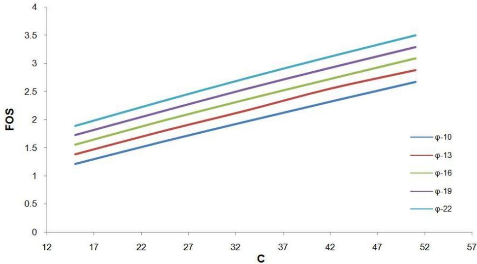
Fig. 3 Relation between stability of slopes and cohesion of soils
