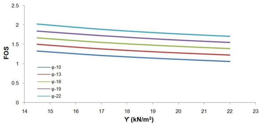
Fig. 1 Relation between stability of slopes and unit weight of soils
