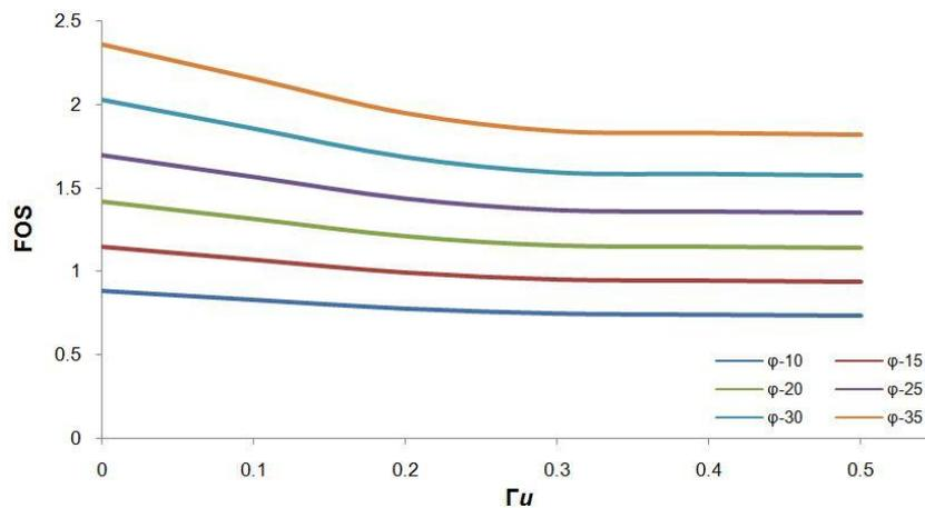
Fig. 10 Relation between stability of slopes and pore water pressure  $\Gamma u$
