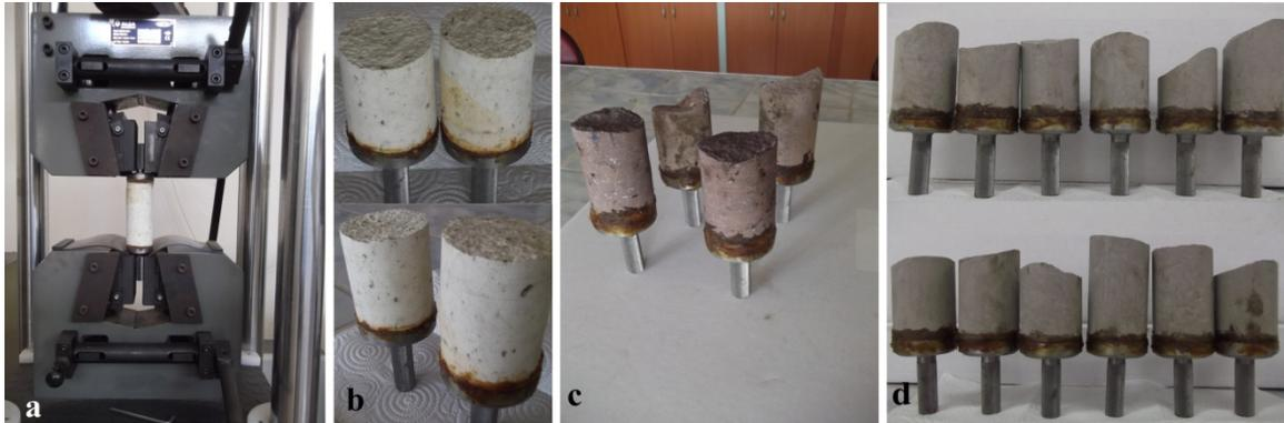
Fig. 14 (a) Direct tensile strength test of cylindrical specimens; (b) failed tuff specimens; (c) failed dacite specimens; (d) failed rocklike specimens
