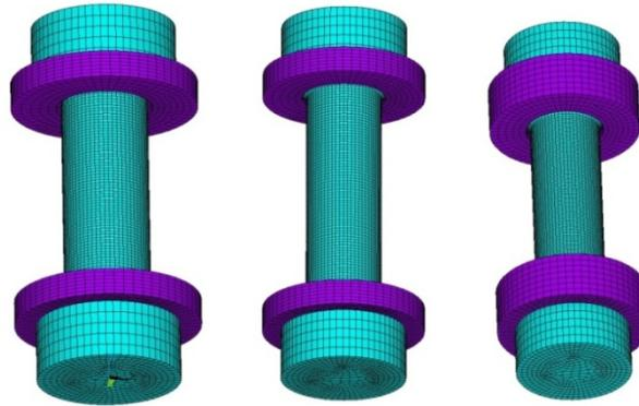
Fig. 2 Some lathed specimens with holding ring models for  $\alpha = 27^\circ$  (left),  $\alpha = 45^\circ$  (mid),  $\alpha = 63^\circ$  (right) conditions
