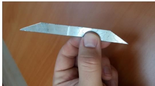
Fig. 8 A reference plate to prepare specimens with the geometry of Model 63-3.2
