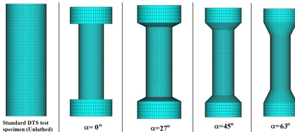
Fig. 1 DTS test specimen models
