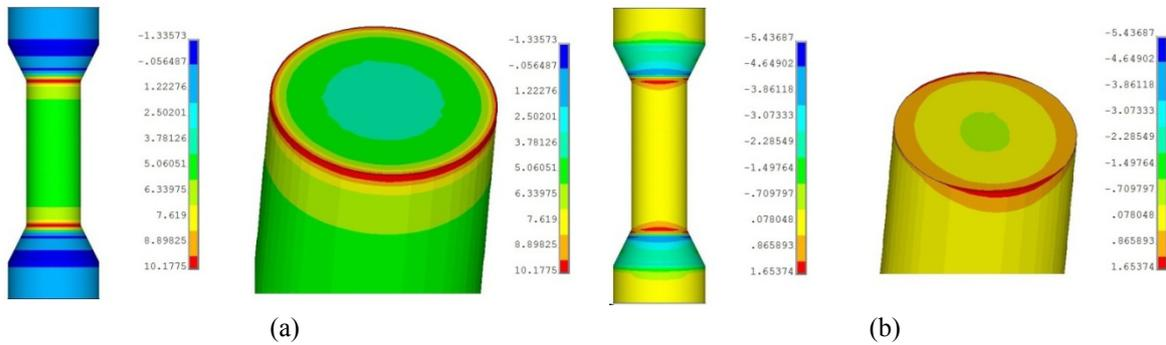
Fig. 5 (a) Vertical stress distribution; (b) horizontal stress distribution in the model with  $\alpha$  angle of  $63^\circ$ , cross-sections of the critical edge (right)
