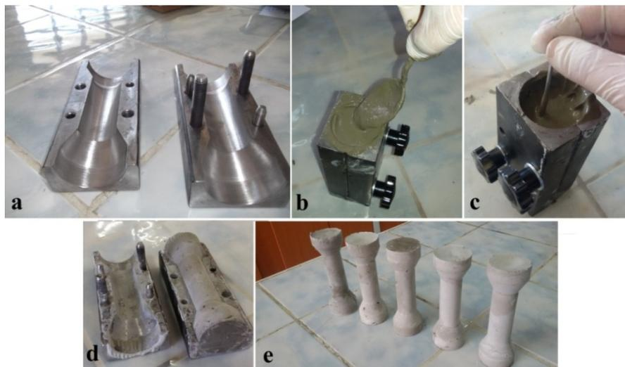
Fig. 11 (a) Mold design; (b) casting mix into the molds; (c) tamping; (d) a specimen in mold; (e) rocklike material specimens with  $\alpha$  angle of  $63^\circ$  and  $d_{\min}$  of 3.2 cm
