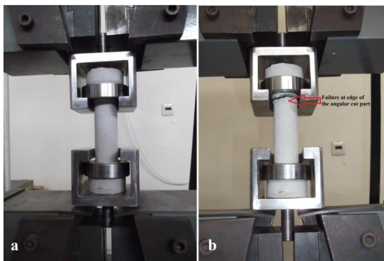
Fig. 13 (a) Lathed specimen testing; (b) failure at the edge of angular cut part
