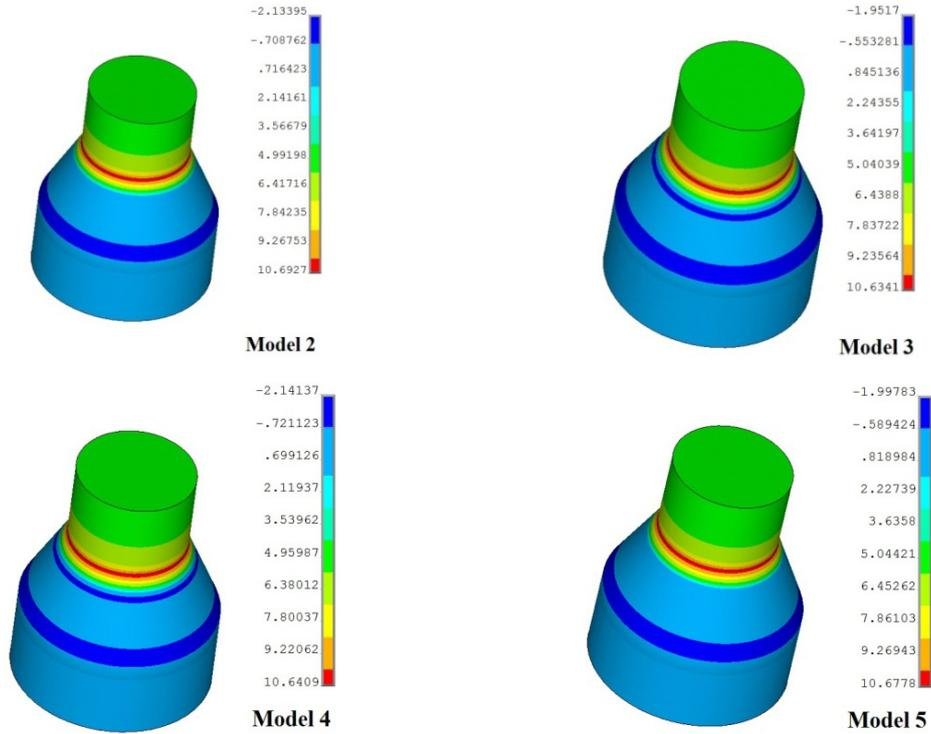
Fig. 7 Major principle stresses in different rock material models with  $\alpha$  of  $63^\circ$  and  $d_{\min}$  of 3.2 cm
