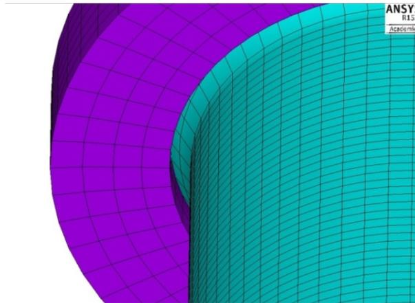
Fig. 3 Steel holding ring touching to the lathed rock sample
