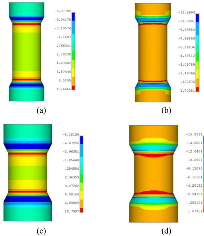
Fig. 6 Stress distributions in long and shortened models with  $\alpha$  angle of  $63^\circ$  and  $d_{\min}$  of 4.3 cm
