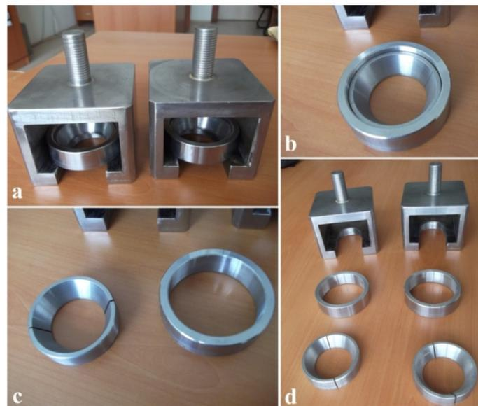
Fig. 12 (a) Steel holder frame cap; (b) and (c) semi-circular ring pair and rings to be inserted semi-circular ring pairs; and (d) steel holder cap setup
