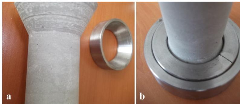
Fig. 10 (a) Specimen prepared to have the cutting geometry of Model 63-3.2; (b) semi-circular pairs contacting to specimens
