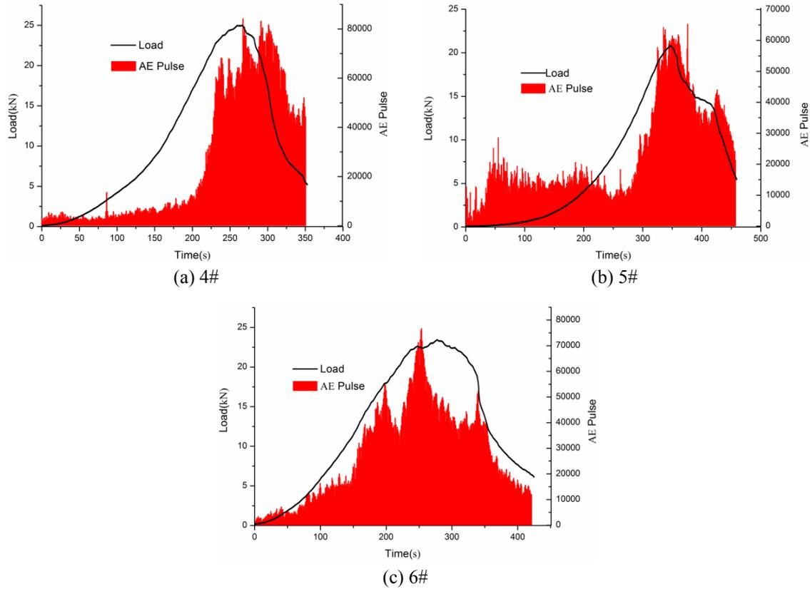
Fig. 4 stress-displacement curves and AE pulse diagram of coal sample 4<sup>#</sup>~6<sup>#</sup>
