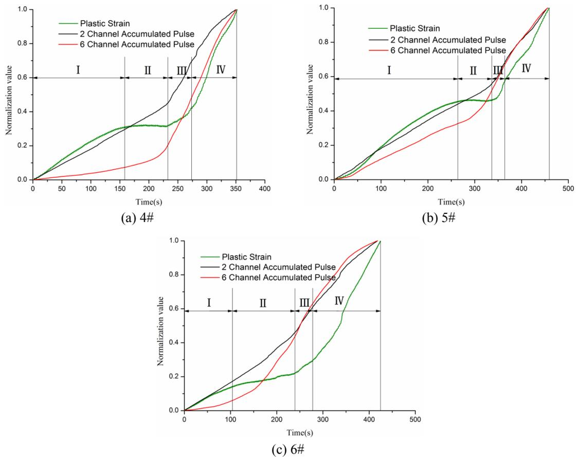
Fig. 5 Summation curves of plastic strain and AE pulse of coal sample 4<sup>#</sup>~6<sup>#</sup>
