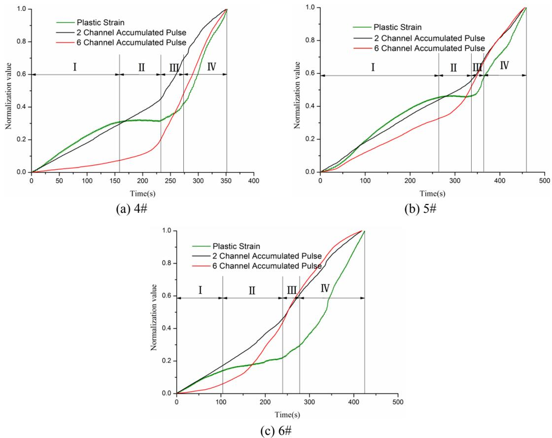
Fig. 5 Summation curves of plastic strain and AE pulse of coal sample 4#~6#
