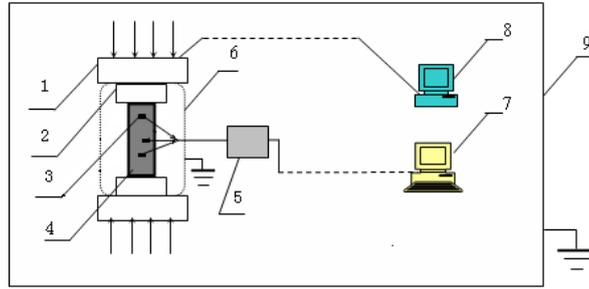
1 – pressure testing machine; 2 – insulated shim; 3 – acoustic-electric sensor;
