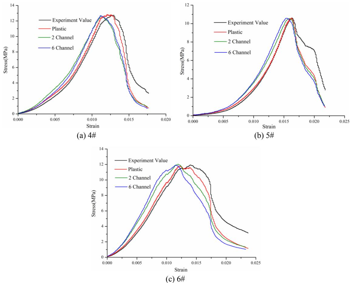
Fig. 6 Contrastive analysis of stress-strain curves
