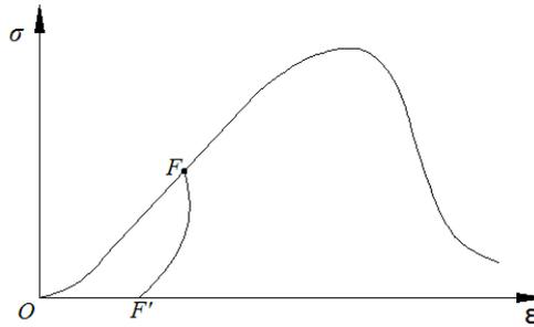
Fig. 1 Stress-strain curve of coal and rock
