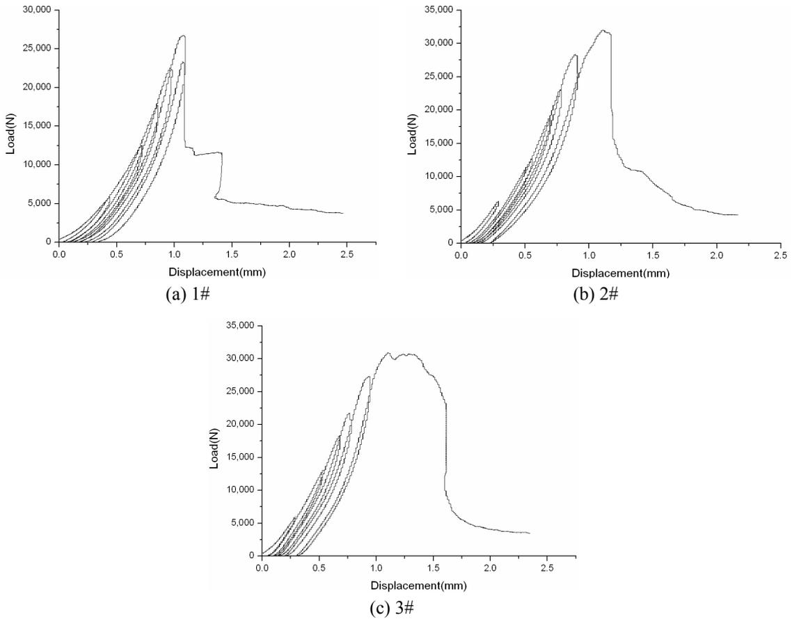
Fig. 3 Stress-displacement curves of coal sample 1<sup>#</sup>~3<sup>#</sup>
