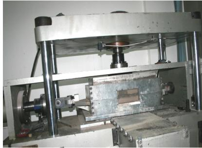
Fig. 2 The large-scale direct shear apparatus (SWJ-200)
