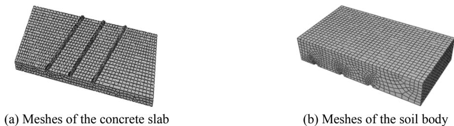
Fig. 12 Finite element meshes used in the numerical modelling
