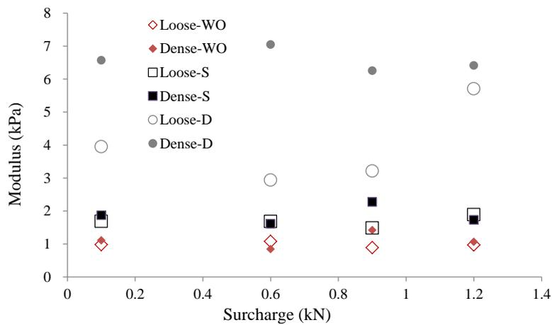
Fig. 10 Changes in the modulus from the number of active tension units under a surcharge in loose and dense sand (Note: WO, S, and D denote bolt without active tension unit, bolt with single active tension unit, and bolt with dual active tension units, respectively)
