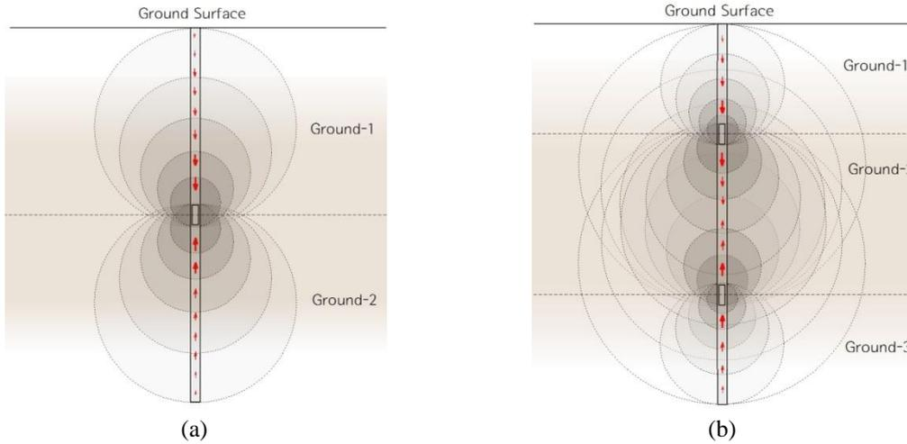
Fig. 2 The load transfer mechanism along the active tension bolt with: (a) a single tension unit; and (b) a dual tension unit
