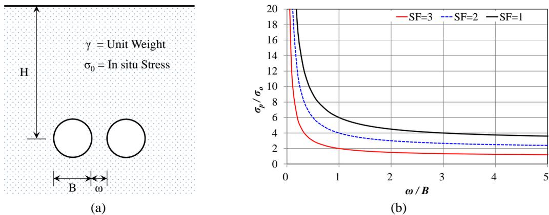
Fig. 11 Design of tunnel pillar: (a) Schematic diagram; (b) Effects of the safety factor on the relationship between  $\omega/B$  and  $\sigma_p/\sigma_0$
