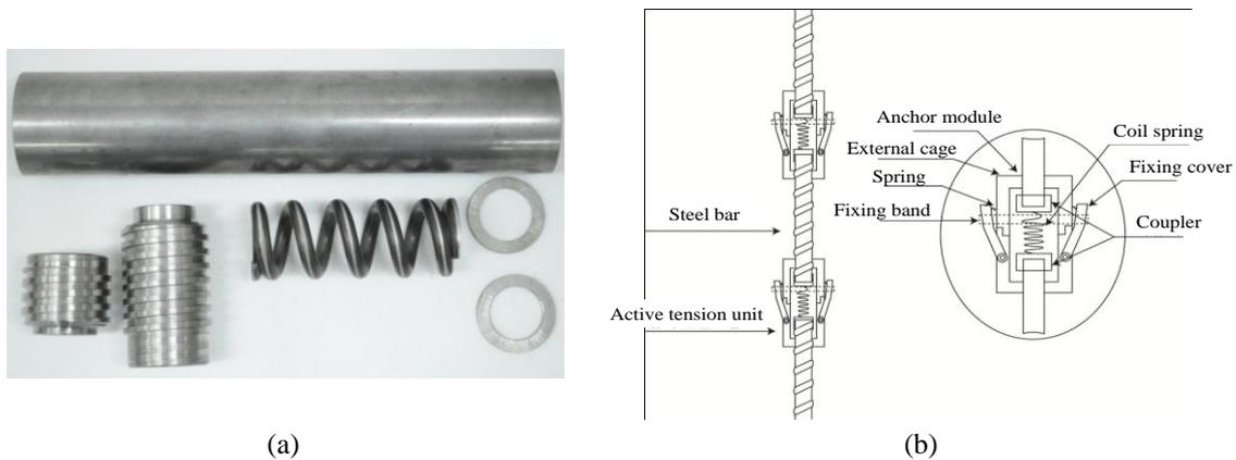
Fig. 4 An active tension unit: (a) components of a tension unit; and (b) the specification of the active tension bolt
