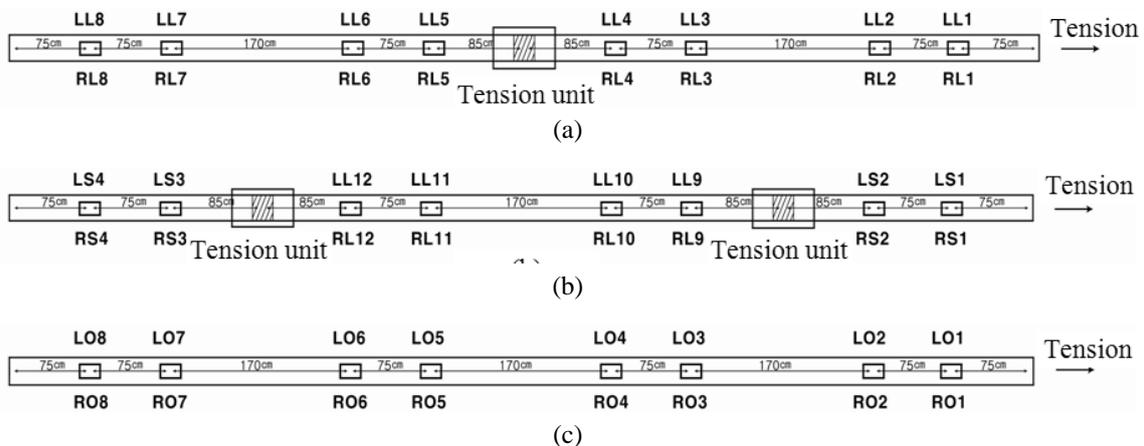
Fig. 8 The location of the strain gauge and the tension unit: (a) a single tension unit; (b) a dual tension 6 unit; and (c) no tension unit
