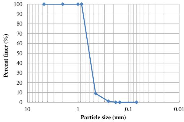
Fig. 6 The particle size distribution of Jumunjin sand
