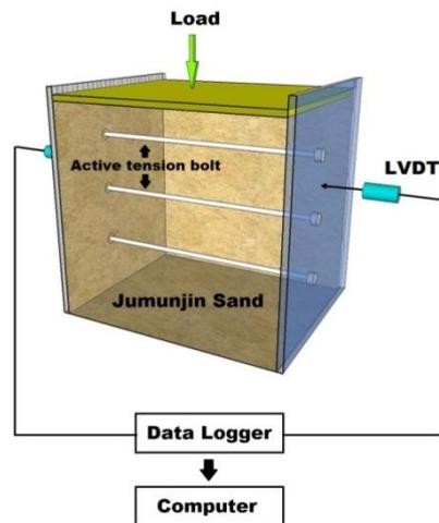
Fig. 13 The experimental setup for investigating the performance of the active tension bolt for pillar reinforcement
