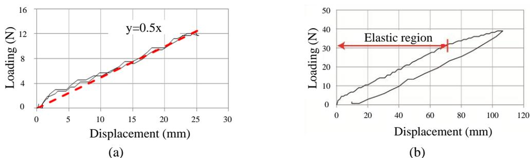
Fig. 5 The load-displacement relationship of the industrial spring: (a) the determination of the spring constant; and (b) the determination of the elastic limit
