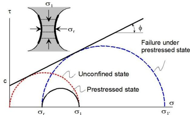
Fig. 12 Changes in the Mohr circle from pillar reinforcement
