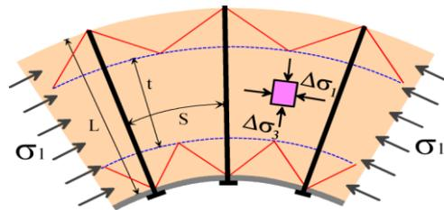
Fig. 3 The stress distribution in the reinforced zone with the active tension bolt
