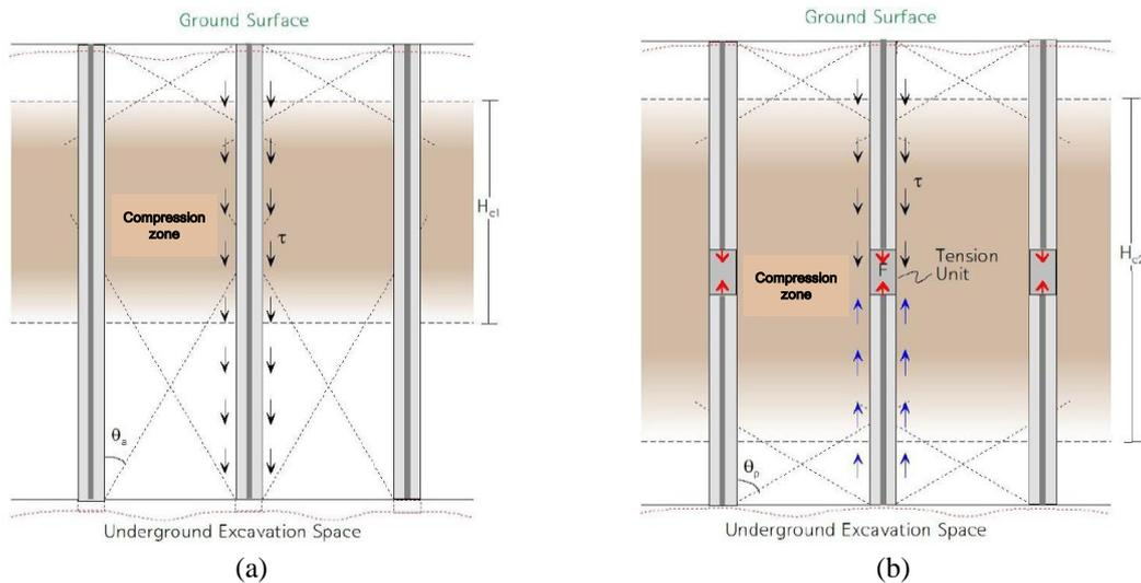
Fig. 1 The thickness of the compressed zone and the direction of mobilized skin friction in: (a) the general bolt system; and (b) the active tension bolt system (note:  $H_{c1}$  is the thickness of the compression zone from a conventional rock bolt system, and  $H_{c2}$  is that from an active tension bolt system)
