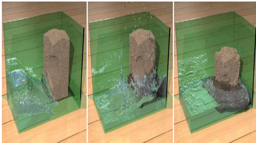
Fig. 9 A moist sand column stands rigidly until a column of water is released. The water percolates through the sand and erodes pieces of the structure
