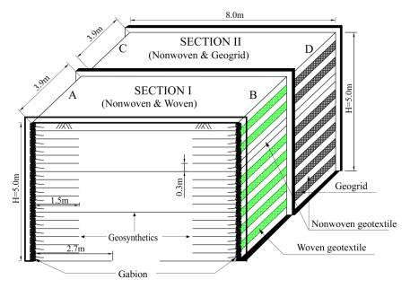
Fig. 1 Schematic diagram of GRS walls
