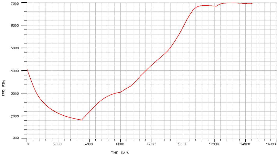
Fig. 5 Reservoir pressure rate
