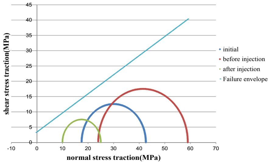
Fig. 11 Stress path for the reservoir for production and injection scenarios
