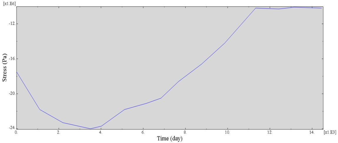
Fig. 10 The minimum principal stresses changes around the well No. 1 during production and injection scenarios
