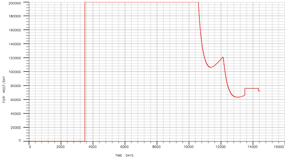
Fig. 6 Well No.1 gas (CO<sub>2</sub>) injection rate
