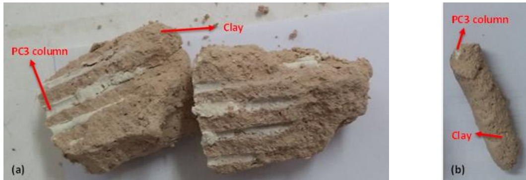
Fig. 5 Views of (a) PC3-Floating -31 columns; and (b) PC3 column after testing
