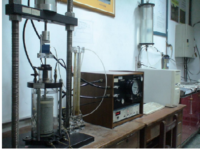
Fig. 3 Dynamic triaxial test
