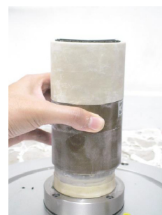
(b) Setting the rubber membrane
