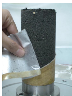
(a) Tearing the paper mold
