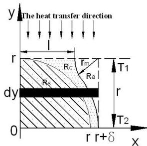
Fig. 3 The unit calculating model
