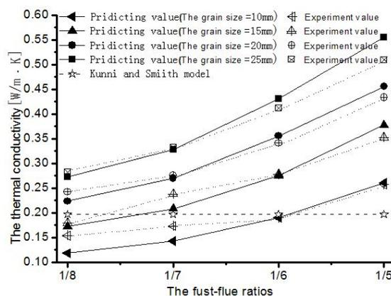
Fig. 5 Comparing with the thermal conductivity by experimental and theory calculating on different particle sizes and cement aggregate ratios
