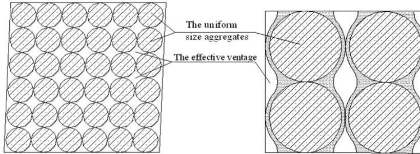
Fig. 2 The simplified skeleton model of high permeability-high strength
