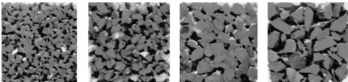
(a) Particle size = 10 mm (b) Particle size = 15 mm (c) Particle size = 20 mm (d) Particle size = 25 mm
