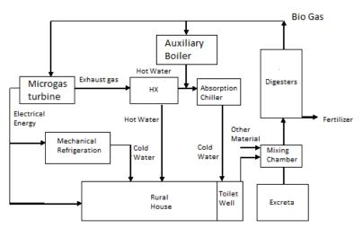
Fig. 5 A schematic of method to supply the energy needed by the rural house using biogas-fueled microturbine in summer
