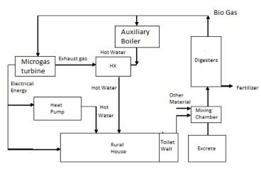
Fig. 6 A schematic of method to supply the energy needed by the rural house using biogas-fueled microturbine in winter
