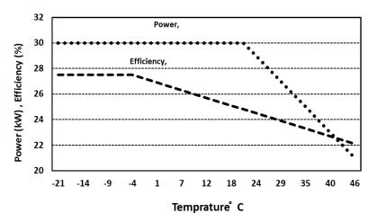
Fig. 7 Changes of e power and  $\eta$  efficiency in Capston C30 microturbine, considering the ambient temperature (www.capstonemicroturbine.com)
