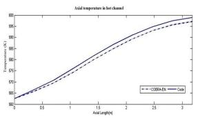
Fig. 7 Axial coolant temperature in hot channel
