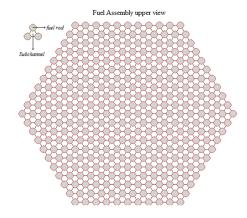
Fig. 5 Top view of subchannel generation
