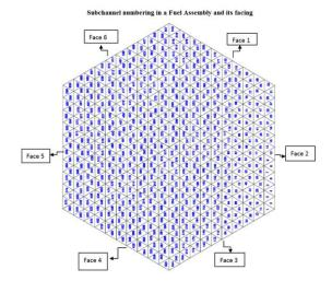
Fig. 18 Fuel Assembly faces, Jointed Channels and FA configuration in one sixth of core (numbering of subchannels is shown)
