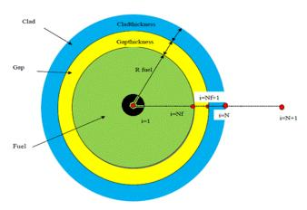
Fig. 4 Fuel pellet with central hole
