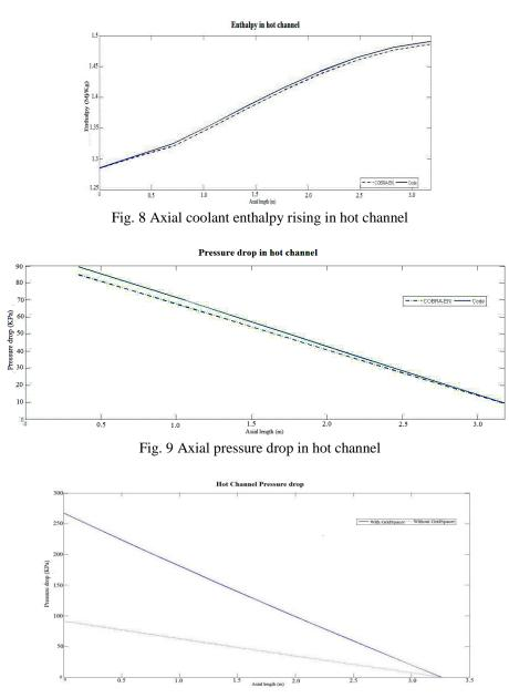
Fig. 10 Axial pressure drop in hot channel
