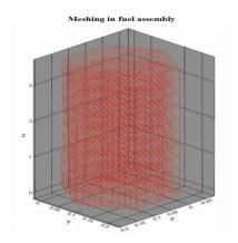
Fig. 6 3D view of subchannel for WWER1000 FA
