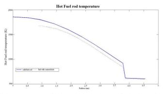
Fig. 16 Radial temperature profile in solid fuel pellet and fuel pellets with central hole
