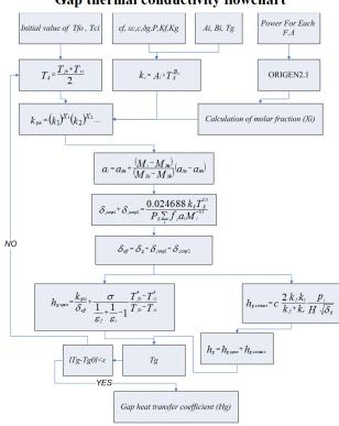
Gap thermal conductivity flowchart
