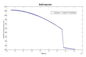
Fig. 13 Radial fuel temperature profiles in finite difference, finite element and analytical methods for pellet with central hole
