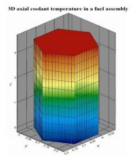
Fig. 17 3D axial coolant temperature in a FA
