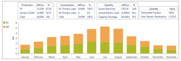
Fig. 8 The share of photovoltaic and wind turbine in electrical production of the hybrid system
