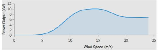
Fig. 5 The power-speed characteristic curve of Generic 10 kW wind turbine
