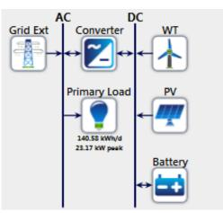
Fig. 1 The proposed HOMER model for a hybrid photovoltaic-wind power system
