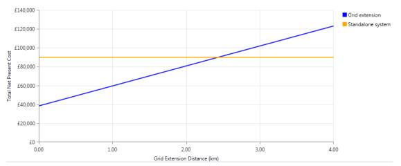
Fig. 9 The grid extension distance versus the total net present cost for a studied hybrid system
