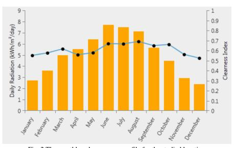
Fig. 2 The monthly solar resource profile for the studied location
