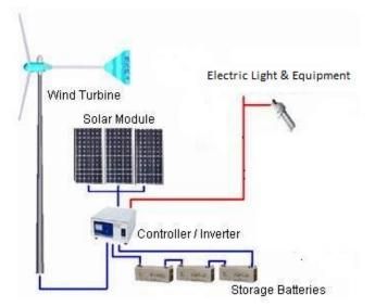
Fig. 6 The proposed model and system structure of the hybrid energy system
