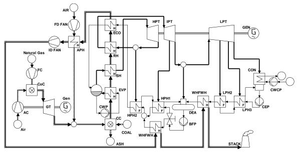
Fig. 2 Schematic diagram of the repowered power plant in Cycle Tempo software interface
