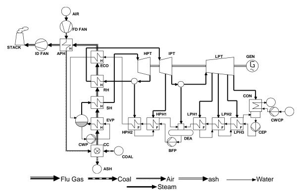
Fig. 1 Schematic diagram of the steam power plant in Cycle Tempo software interface
