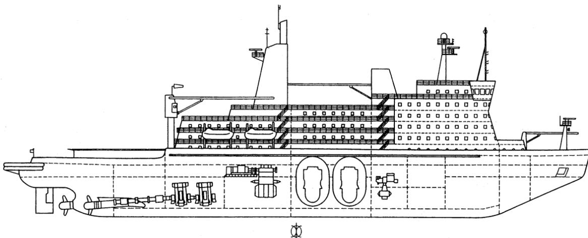
Fig. 3 Schematic of the place of the MRX put in the middle part of the icebreaker ship adapted from Kusunoki (2000)
