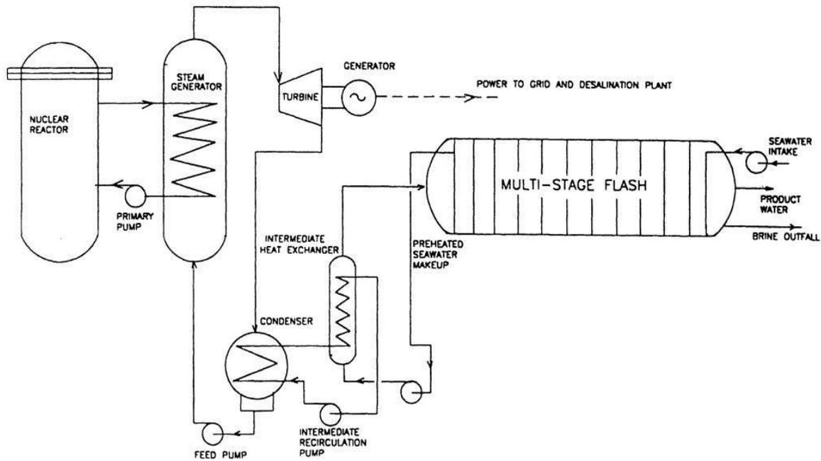
Fig. 1 Schematic illustration of a simple desalination nuclear reactor circuit (Majumdar 2002)
