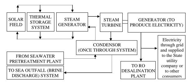
Fig. 2 Block diagram for solar power plant in Copper industry
