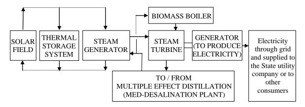
Fig. 4 Block diagram (modified) for the solar power plant in Copper industry
