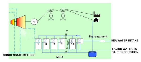
Fig. 6 Flow diagram (modified) showing MED desalination plant in Copper industry
