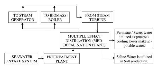
Fig. 5 Block diagram (modified) for desalination plant in Copper industry
