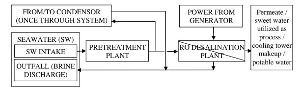
Fig. 3 Block diagram for RO Desalination plant in Copper industry
