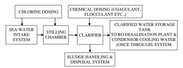
Fig. 1 Block diagram for seawater pretreatment plant in Copper industry.
