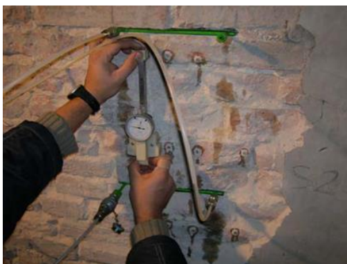
(a) typical double flat-jack test (Bartoli et al. 2008)
