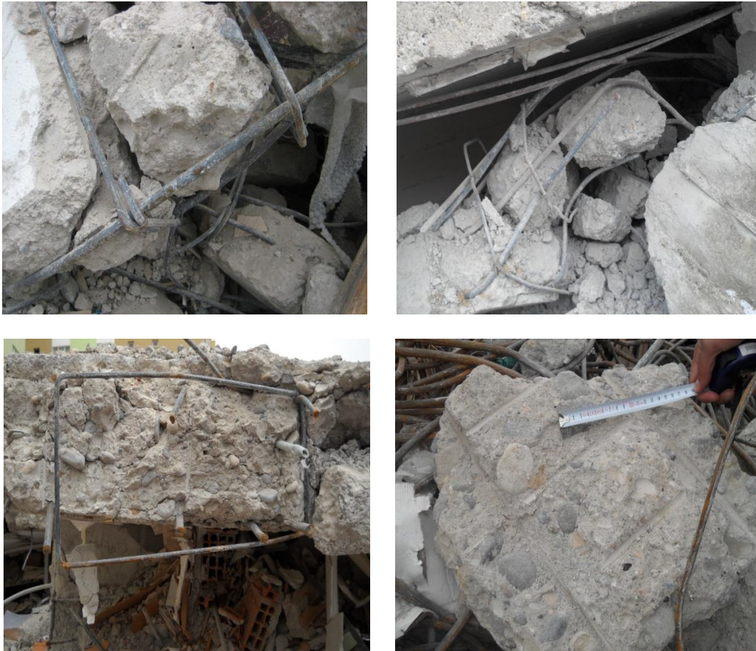
Fig. 20 Poor quality concrete at various buildings
