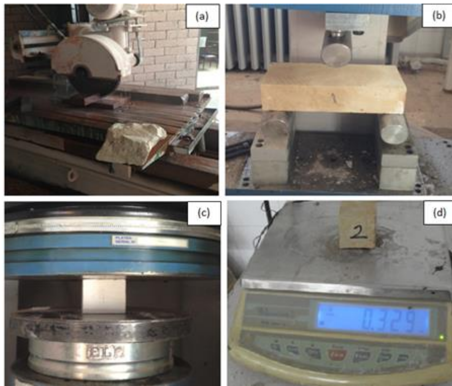
Fig. 11 (a) Preparation of the specimens, (b) Three-point bending test, (c) Compression test, (d) Density test
