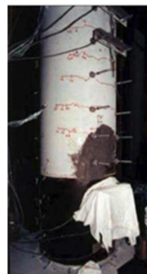
Fig. 12 Comparison of FEM with the experiment (Hewes and Priestley 2002): sample with aspect ratio of 6
