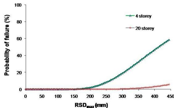
Fig. 14 Fragility curves for collapse of case study soft-storey precast columns
