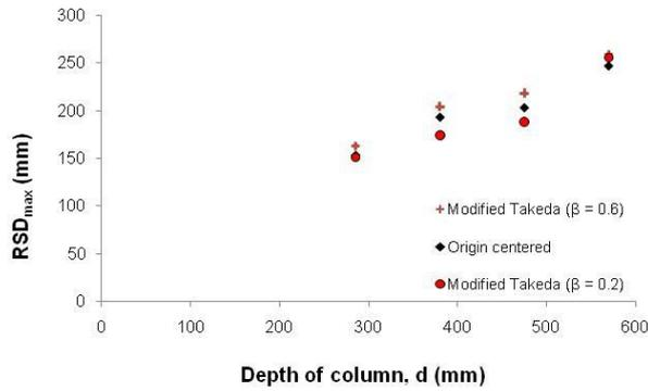
Fig. 10 Correlation of RSD<sub>max</sub> with column depth for 5 % probability of failure
