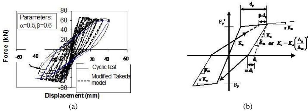
Fig. 7 (a) Recorded and calibrated hysteresis curves (Rodsini 2007) (b) Modified Takeda model (Carr 2008)
