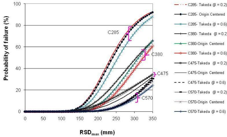
Fig. 9 Comparison of fragility curves for different column dimensions with same aspect ratio (M7 earthquake scenario on class D site)
