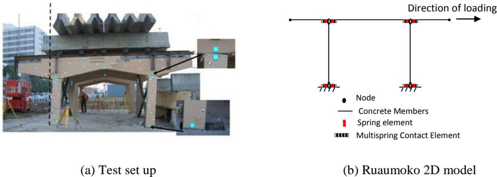
Fig. 5 Test set up and Ruaumoko 2D model of precast soft-storey structure
