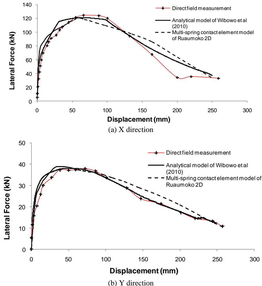
Fig. 6 Comparison of force-displacement behaviour (with ground floor slab isolated from column)
