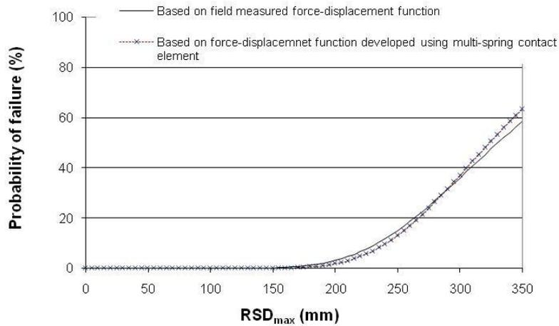
Fig. 8 Fragility curves based on force-displacement relationships obtained from field test and from program Ruaumoko in X direction
