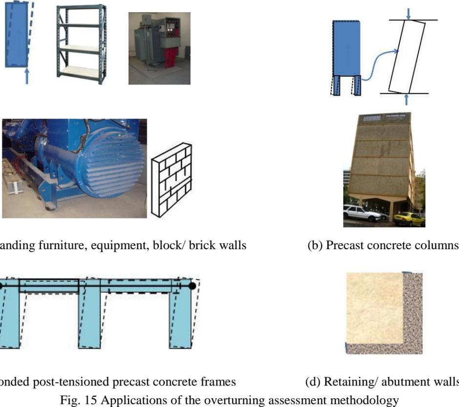
Fig. 15 Applications of the overturning assessment methodology
