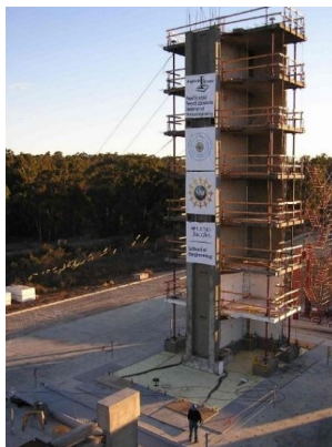
Fig. 15 A seven-story wall building tested at UCSD
