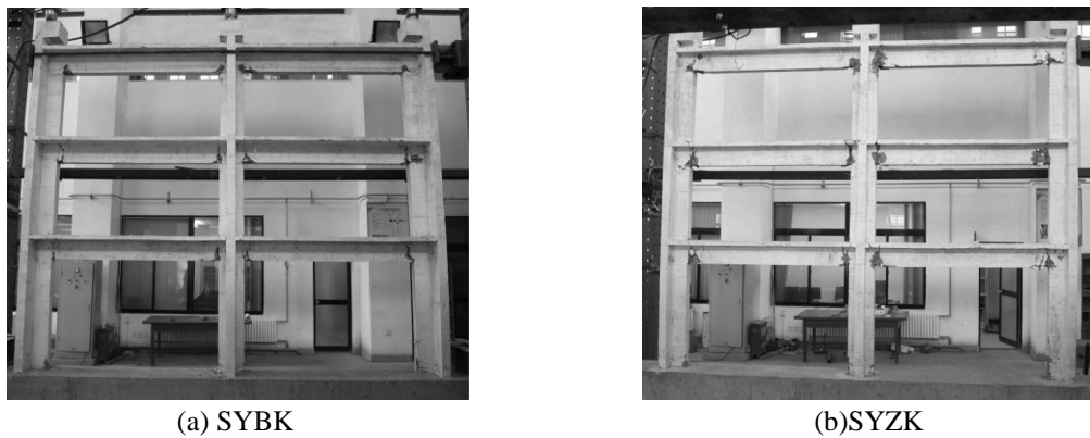
Fig.9 Failure patterns of whole frames
