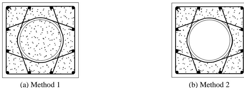
Fig. 3 Concrete area used for calculation of volumetric transverse reinforcement ratio
