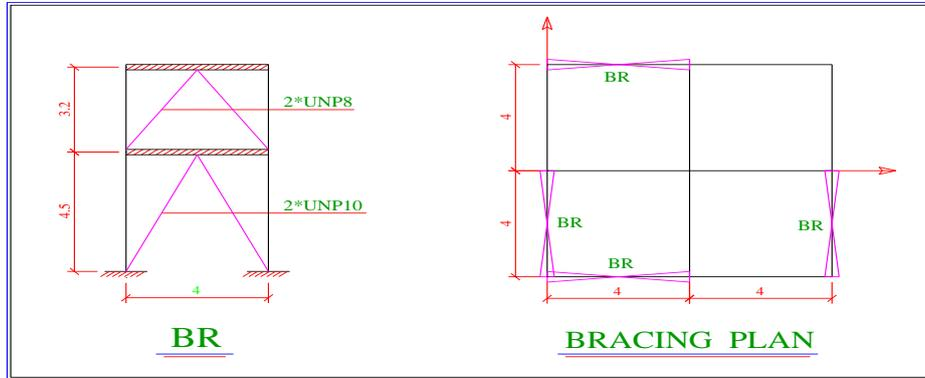
Fig. 3 Bracing plan and Bracing elevation of a commercial building, (UNP represents the cross-section of the braces' profile)
