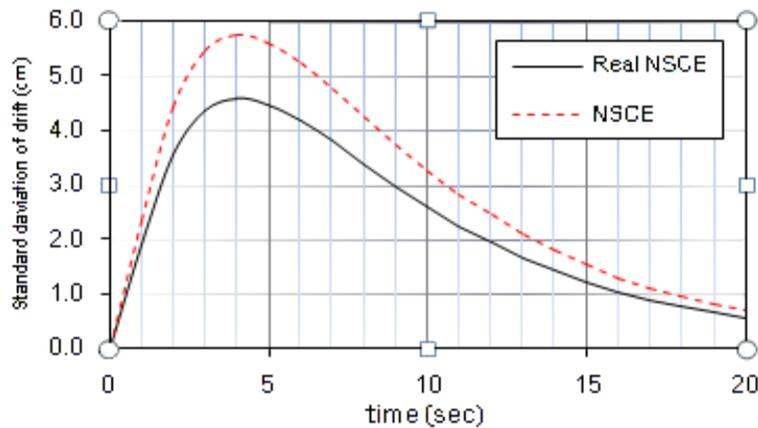
Fig. 6 Standard deviation of inter-story drift for the non-stationary critical excitation
