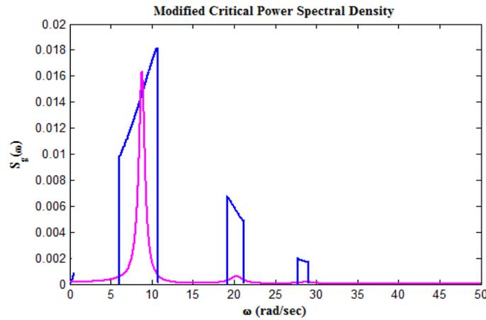
Fig. 2 Modified form of the critical excitation PSD function
