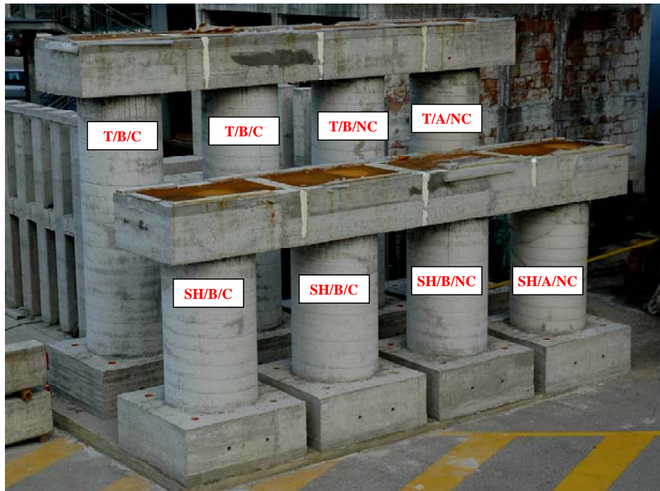
Fig. 1 Experimental models: Tall (T) and Short (SH) piers, Corroded (C) and not corroded (NC) reinforcement, type A and type B of micro concrete
