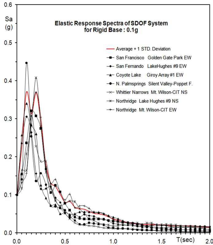
Fig. 2 Response spectra of 7 earthquake records (0.1 g)
