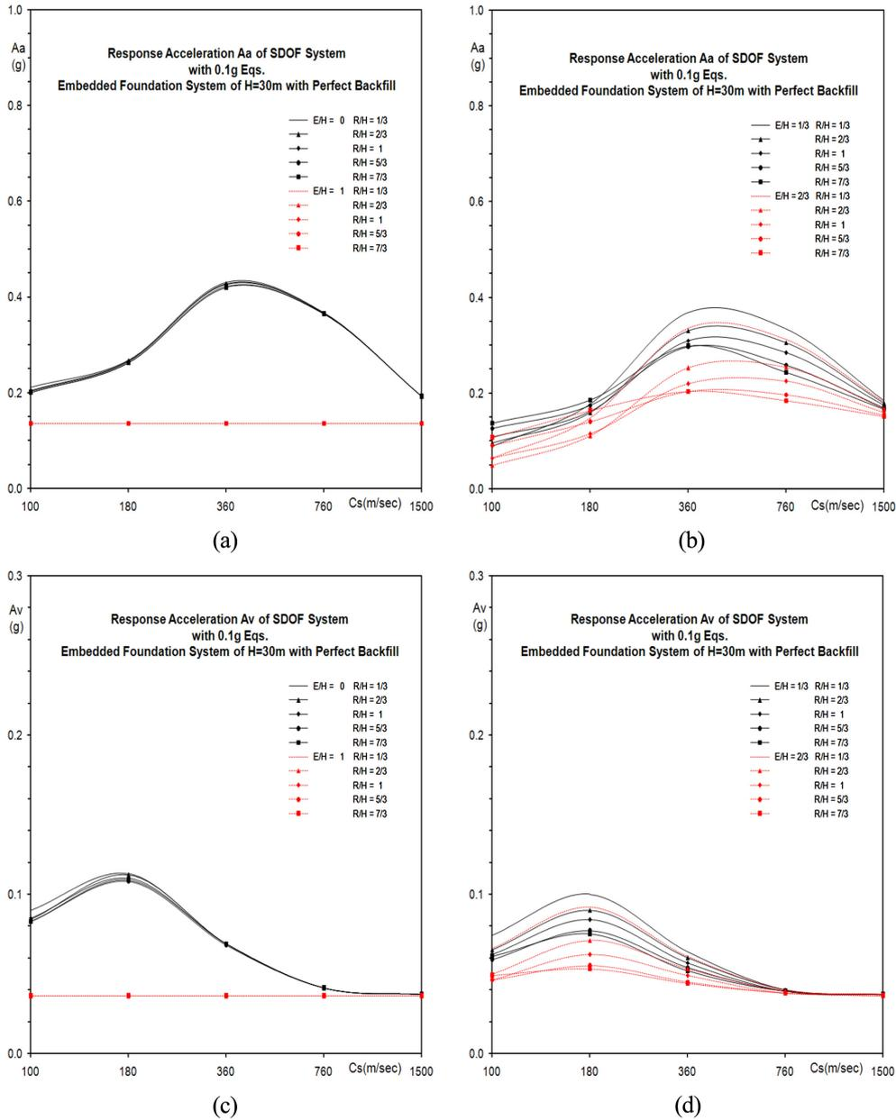
Fig. 3 Response accelerations of  $A_a$  and  $A_v$  with perfect backfill: (a)  $A_a$  in the case of  $E/H=0$  and 1, (b)  $A_a$  in the case of  $E/H=1/3$  and  $2/3$ , (c)  $A_v$  in the case of  $E/H=0$  and 1 and (d)  $A_v$  in the case of  $E/H=1/3$  and  $2/3$
