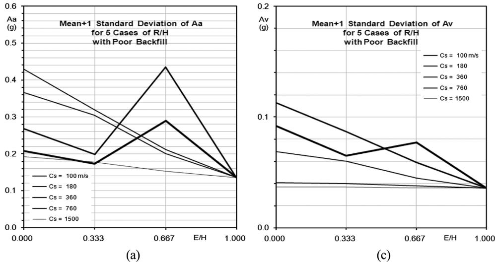
Fig. 6 Mean+SD of  $A_a$  and  $A_v$  for 5 cases of  $R/H$  with poor backfill: (a) Mean+SD of  $A_a$  and (b) Mean+SD of  $A_v$
