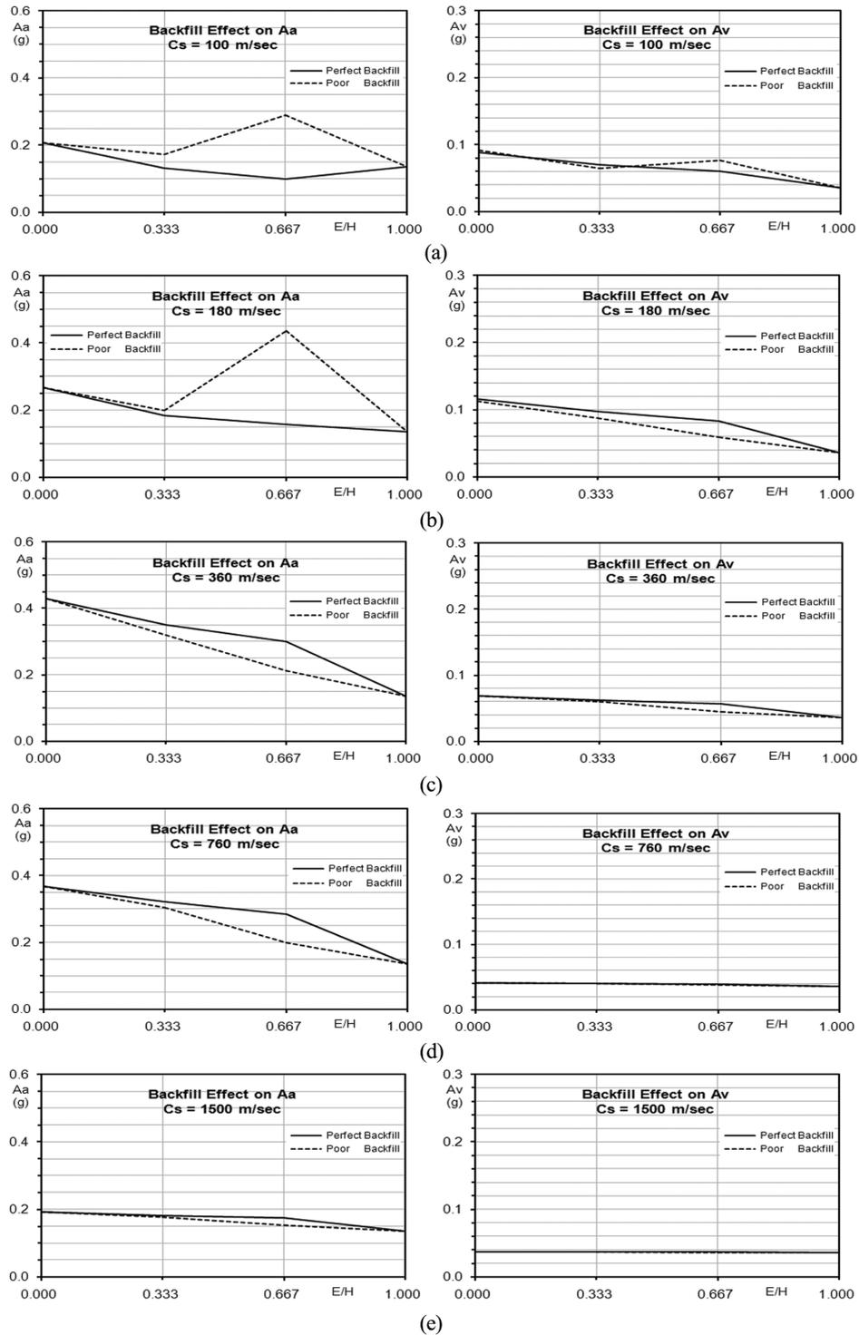
Fig. 7 Backfill effect on the response acceleration of  $A_a$  and  $A_v$ : (a)  $C_s=100$  m/s, (b)  $C_s=180$  m/s, (c)  $C_s=360$  m/s, (d)  $C_s=760$  m/s and (e)  $C_s=1500$  m/s
