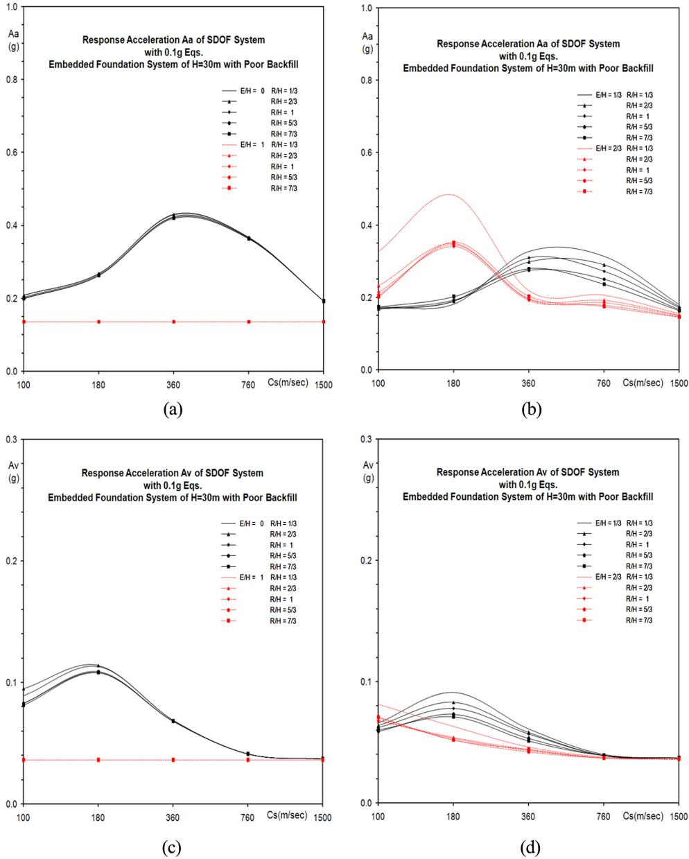
Fig. 5 Response accelerations of  $A_a$  and  $A_v$  with poor backfill: (a)  $A_a$  in the case of  $E/H=0$  and 1, (b)  $A_a$  in the case of  $E/H=1/3$  and  $2/3$ , (c)  $A_v$  in the case of  $E/H=0$  and 1 and (d)  $A_v$  in the case of  $E/H=1/3$  and  $2/3$
