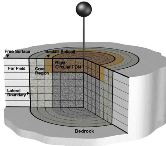
Fig. 1 Pseudo-3D finite-element model
