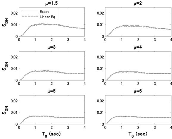
Fig. 11 Normalized displacement spectra -Earthquake  $S_{//0}$ , Soil I-
