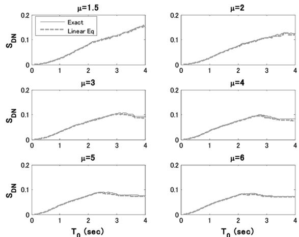
Fig. 10 Normalized displacement spectra -Earthquake  $S_{10}$ , Soil III-
