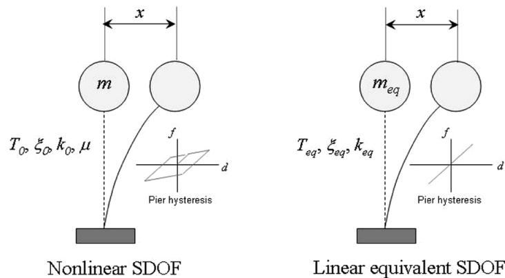
Fig. 1 Nonlinear SDOF simplified into an equivalent SDOF system
