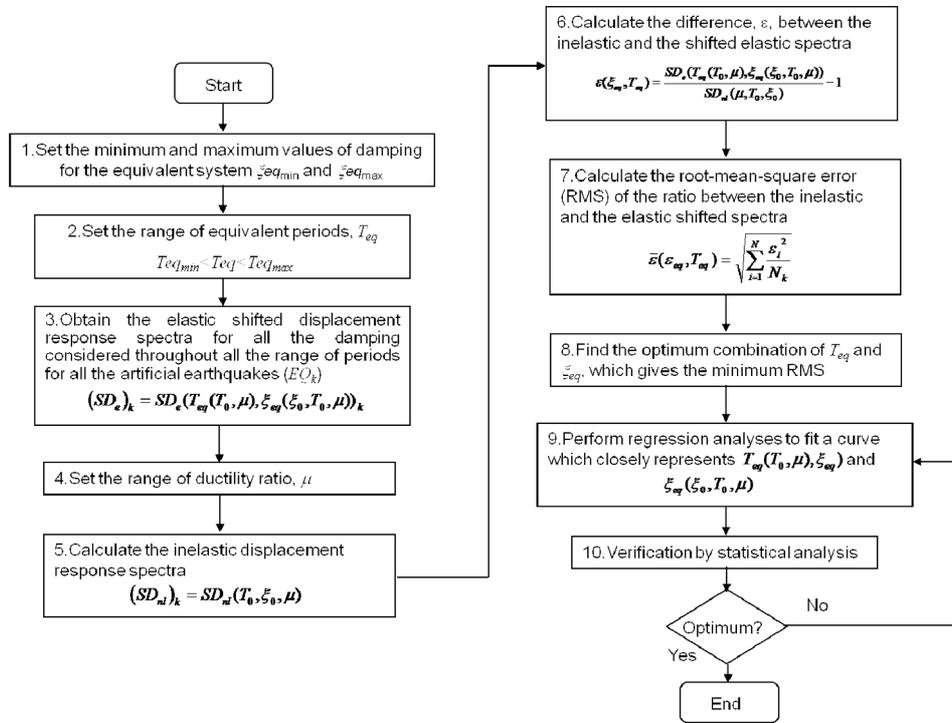
Fig. 3 Procedure followed to derive expressions for the equivalent properties
