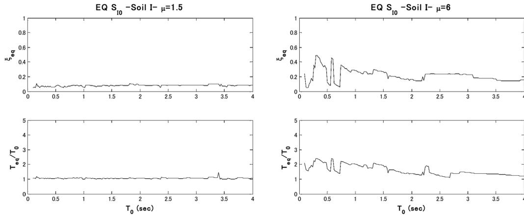
Fig. 8 Optimal period shift and equivalent damping derived from the minimum RMS error
