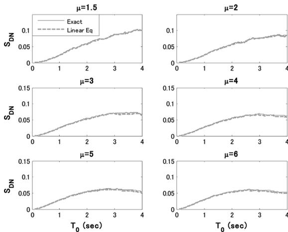
Fig. 9 Normalized displacement spectra -Earthquake  $S_{10}$ , Soil I-
