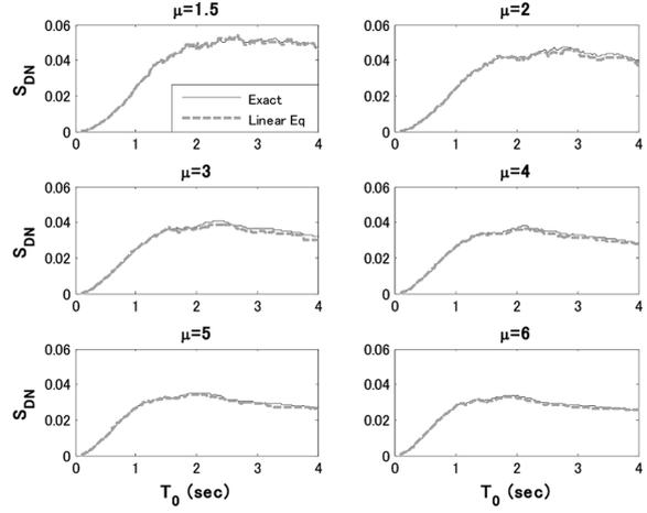
Fig. 12 Normalized displacement spectra -Earthquake  $S_{//0}$ , Soil III-
