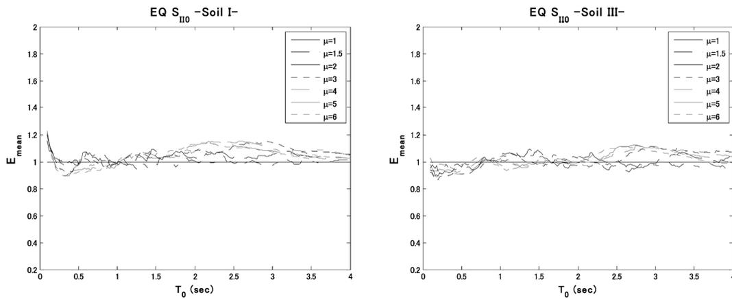
Fig. 15 Mean approximate to exact displacement ratios -Earthquake  $S_{110}$ -
