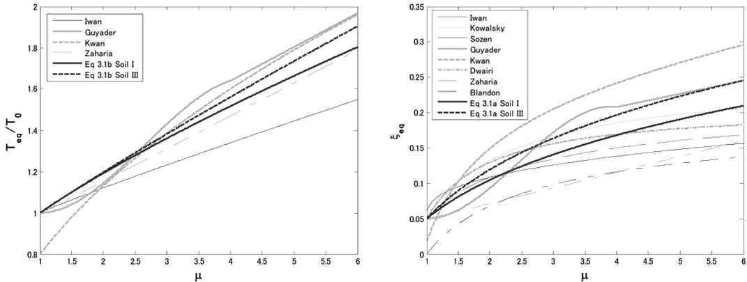
Fig. 13 Comparison of the proposed  $T_{eq}/T_0$  and  $\xi_{eq}$  with other linearization models
