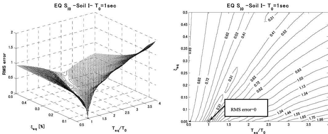
Fig. 7 Minimum SMS error in the region  $RMS\ error - \xi_{eq} - T_{eq}/T_0$
