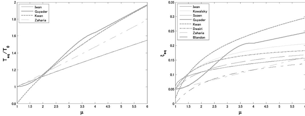
Fig. 2 Comparison of  $T_{eq}/T_0$  and  $\xi_{eq}$  for different equivalent linearization models
