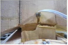
(b) Tensile failure of the tenon-neck Fig. 8 Failure modes of the mortise-tenon joints
