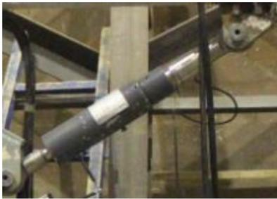
Fig. 3 Sketch of viscous damper
