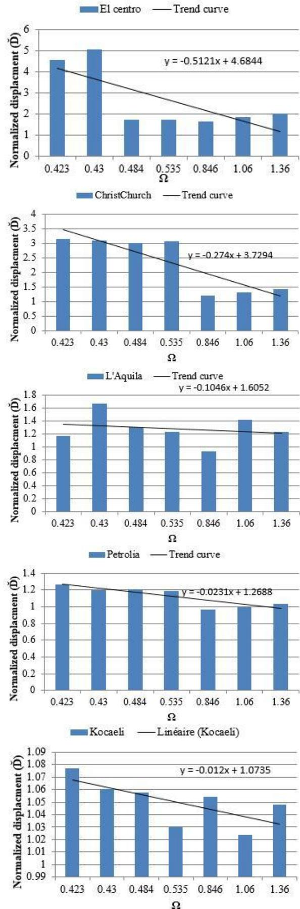
Fig. 5 Effect of frequency ratio on normalized displacement
