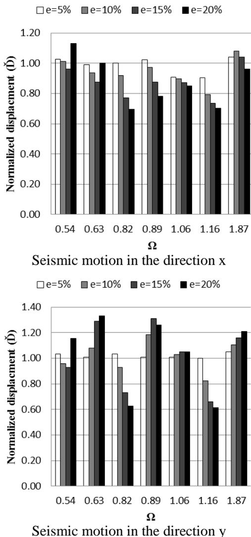
Fig. 7 Effect of frequency ratio on normalized displacement, by applying the conventional calculation of accidental eccentricity e
