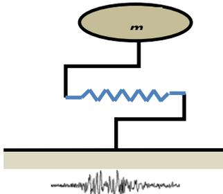
Fig. 1 (a) The spring mass system
