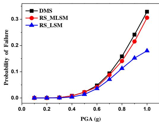
Fig. 6 Comparison of fragility curves for SDOF system (allowable displacements of 0.812 m)
