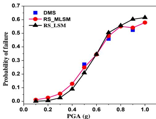
Fig. 9 Comparison of fragility curves of the considered building frame at IO level
