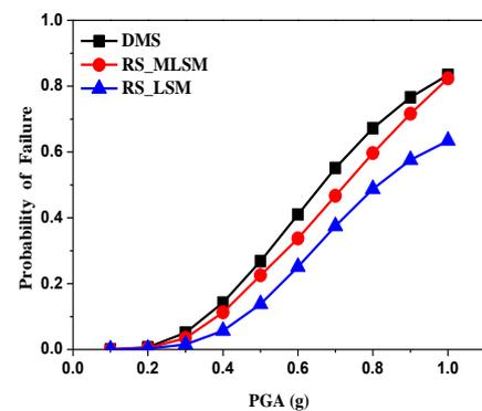
Fig. 5 Comparison of fragility curves for SDOF system (allowable displacements of 0.406 m)
