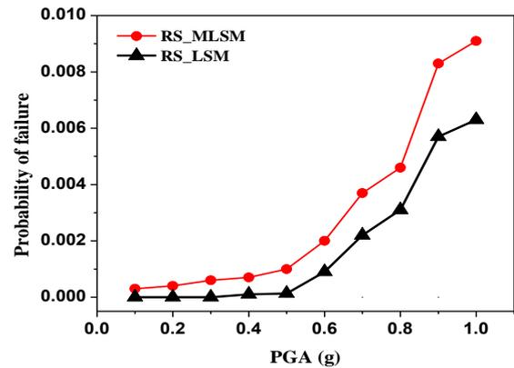
Fig. 11 Comparison of fragility curves of the considered building frame at CP level
