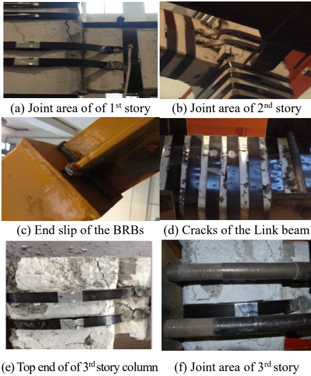
Fig. 6 Failure mode and crack of RCF1
