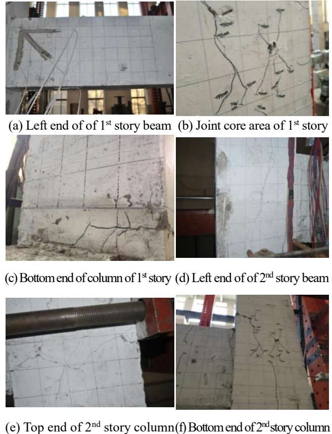
Fig. 5 Failure mode and cracks of specimen RCF1
